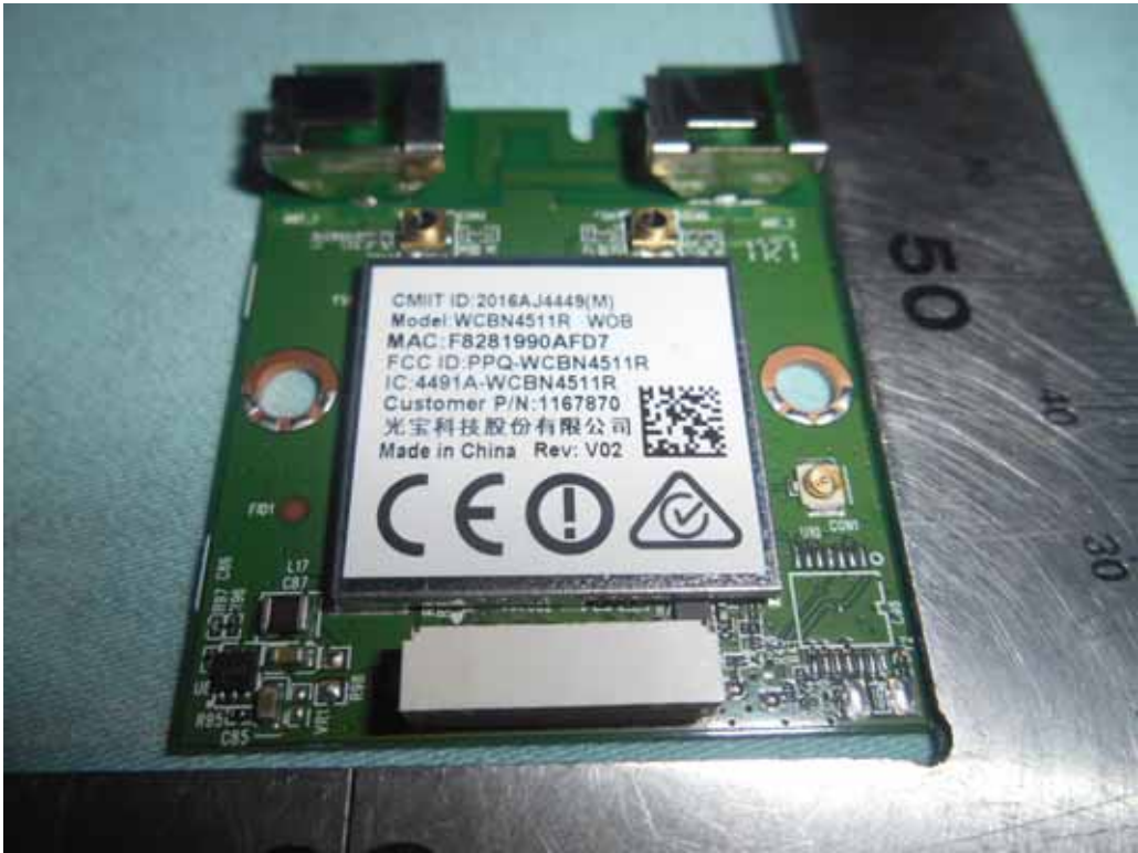
FIGURE 9 LED LCD TV (M/N: 65H8D) RF BOARD (COMPONENT SIDE)
