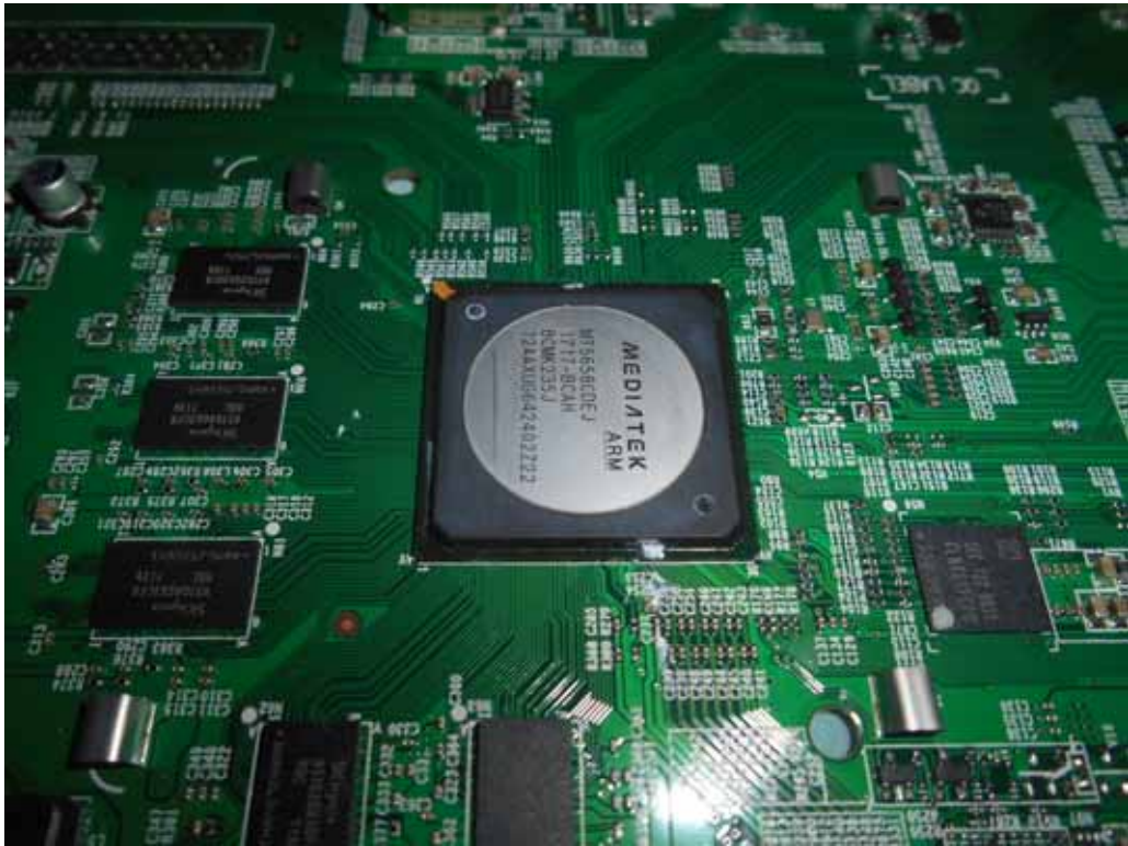
FIGURE 5 LED LCD TV (M/N: 65H8D) CHIP AND CRYSTAL ON MAIN BOARD
