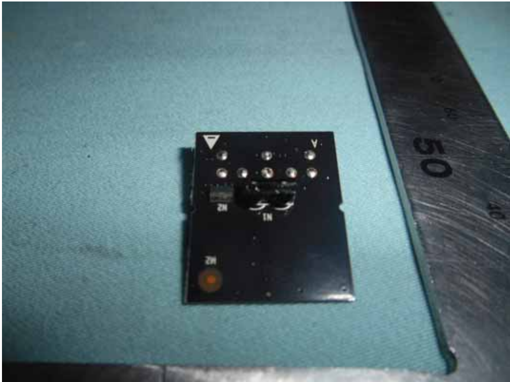
FIGURE 19 LED LCD TV (M/N: 65H8D) IR BOARD (SOLDERED SIDE)
