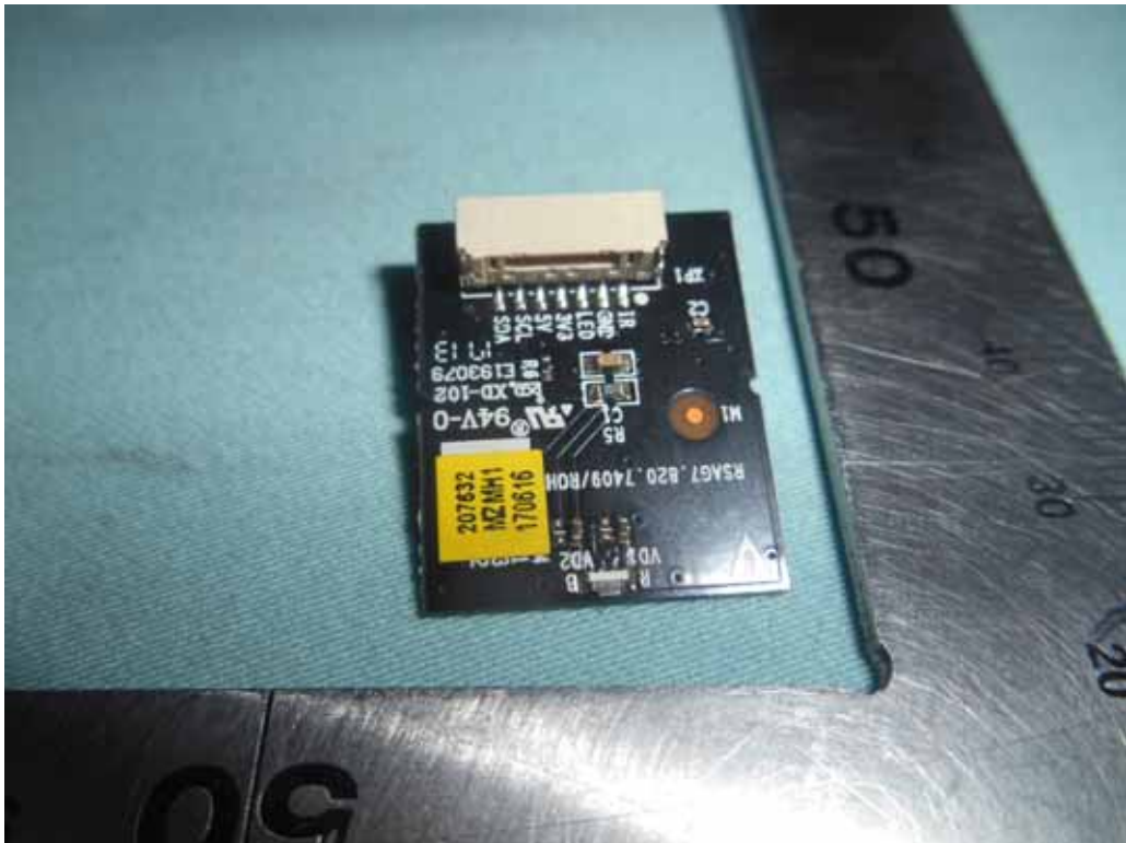
FIGURE 18 LED LCD TV (M/N: 65H8D) IR BOARD (COMPONENT SIDE)
