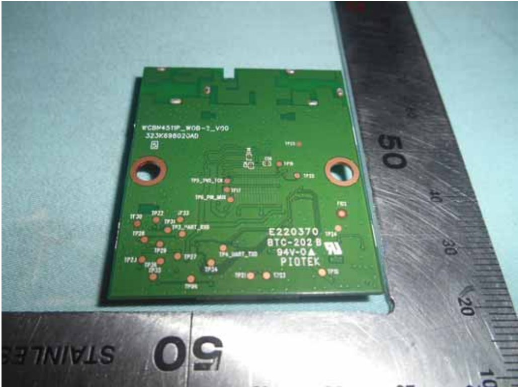
FIGURE 10 LED LCD TV (M/N: 65H8D) RF BOARD (SOLDERED SIDE)
