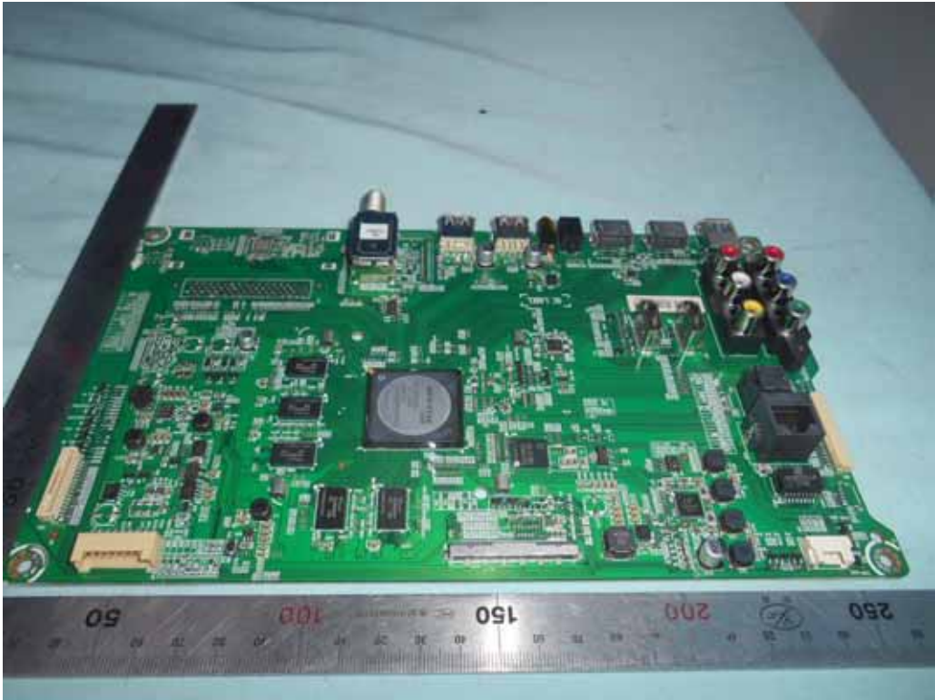
FIGURE 3 LED LCD TV (M/N: 65H8D) MAIN BOARD (COMPONENT SIDE)
