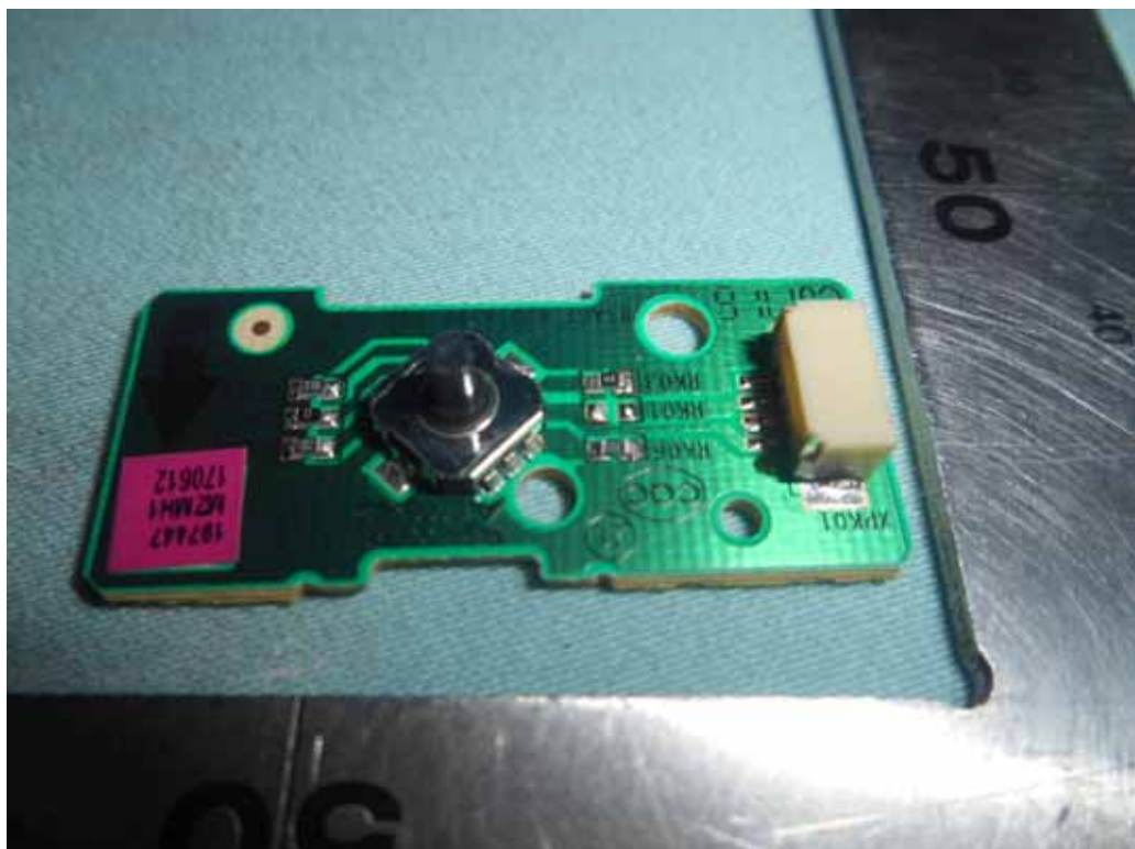
FIGURE 16 LED LCD TV (M/N: 65H8D) KEY BOARD (COMPONENT SIDE)
