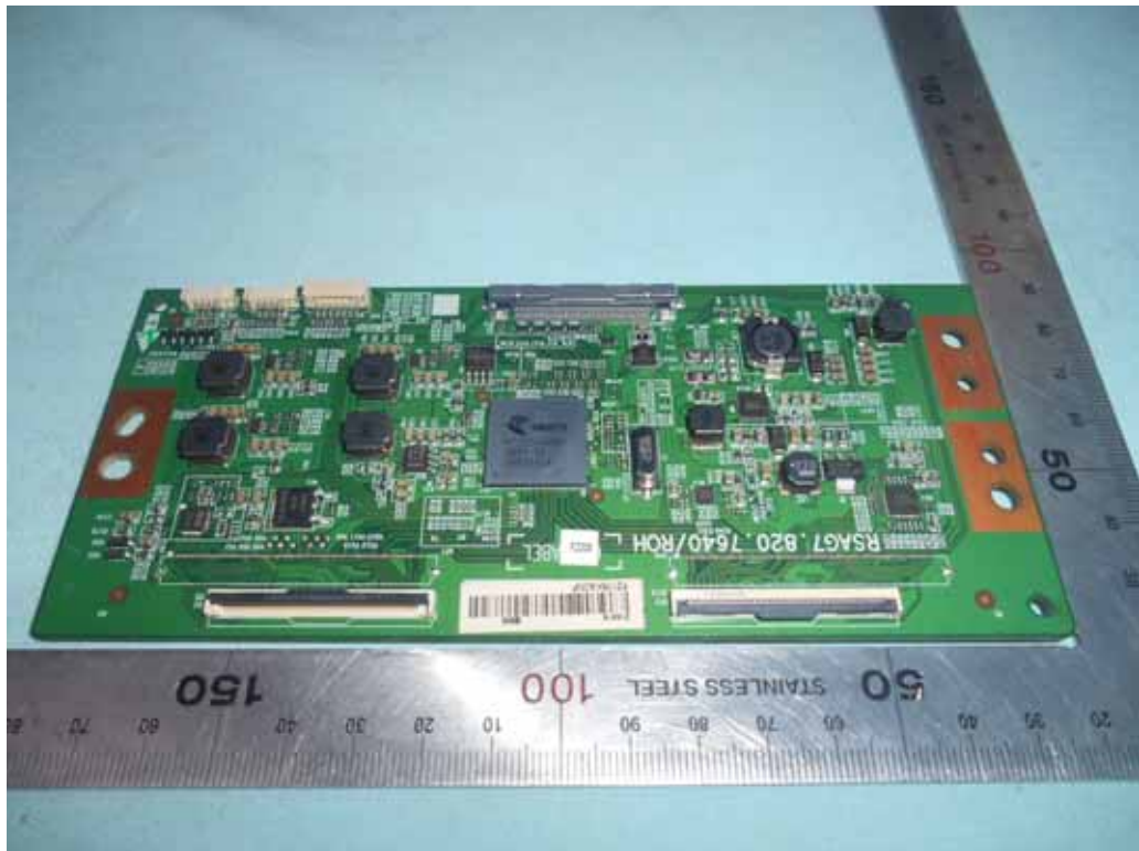
FIGURE 13 LED LCD TV (M/N: 65H8D) PANEL CONTROL BOARD (COMPONENT SIDE)
