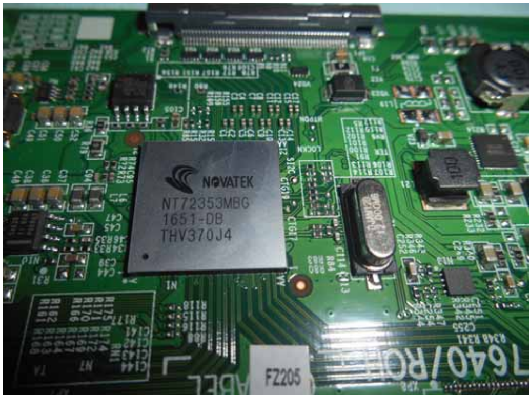
FIGURE 15 LED LCD TV (M/N: 65H8D) CHIP ON PANEL CONTROL BOARD
