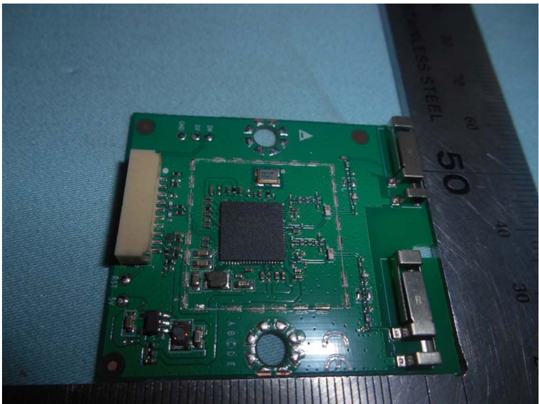
FIGURE 16 LED LCD TV (M/N: LC-50N8002U) RF BOARD COVER REMOVED
