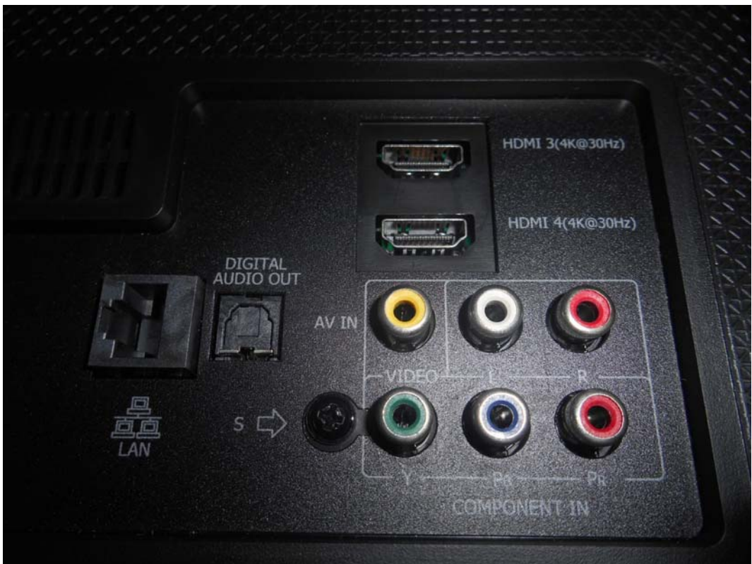
FIGURE 4 LED LCD TV (M/N: 50H8D) PORTS #2
