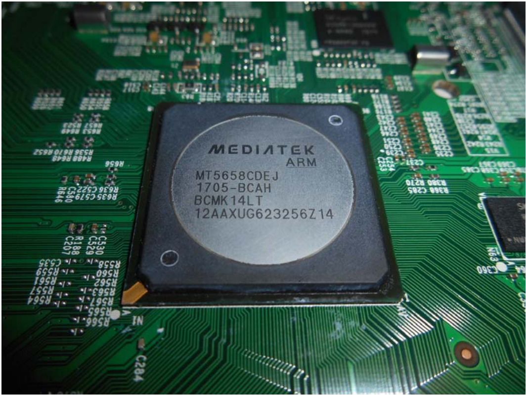
FIGURE 5 LED LCD TV (M/N: 50H8D) CRYSTAL & CHIP ON MAIN BOARD
