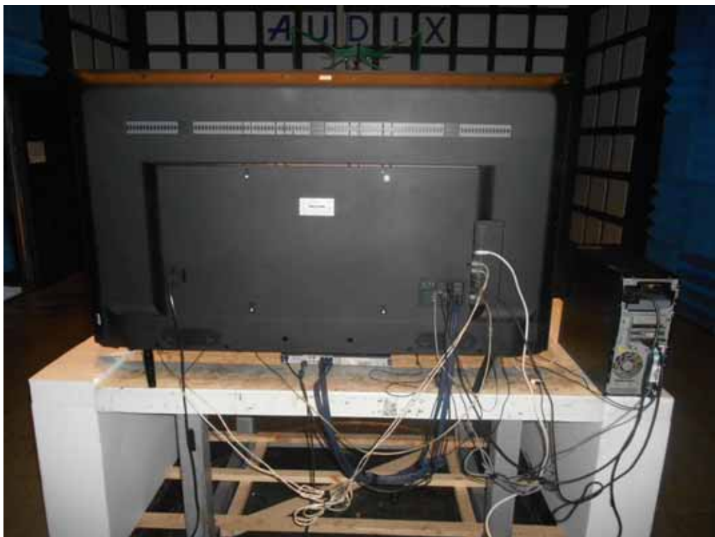
BACK VIEW OF RADIATED EMISSION TEST (BELOW 1GHZ)
