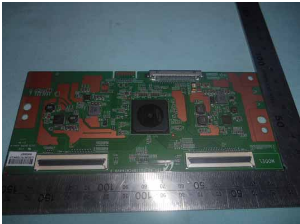
FIGURE 13 LED LCD TV (M/N: 65H7D) PANEL CONTROL BOARD (COMPONENT SIDE)
