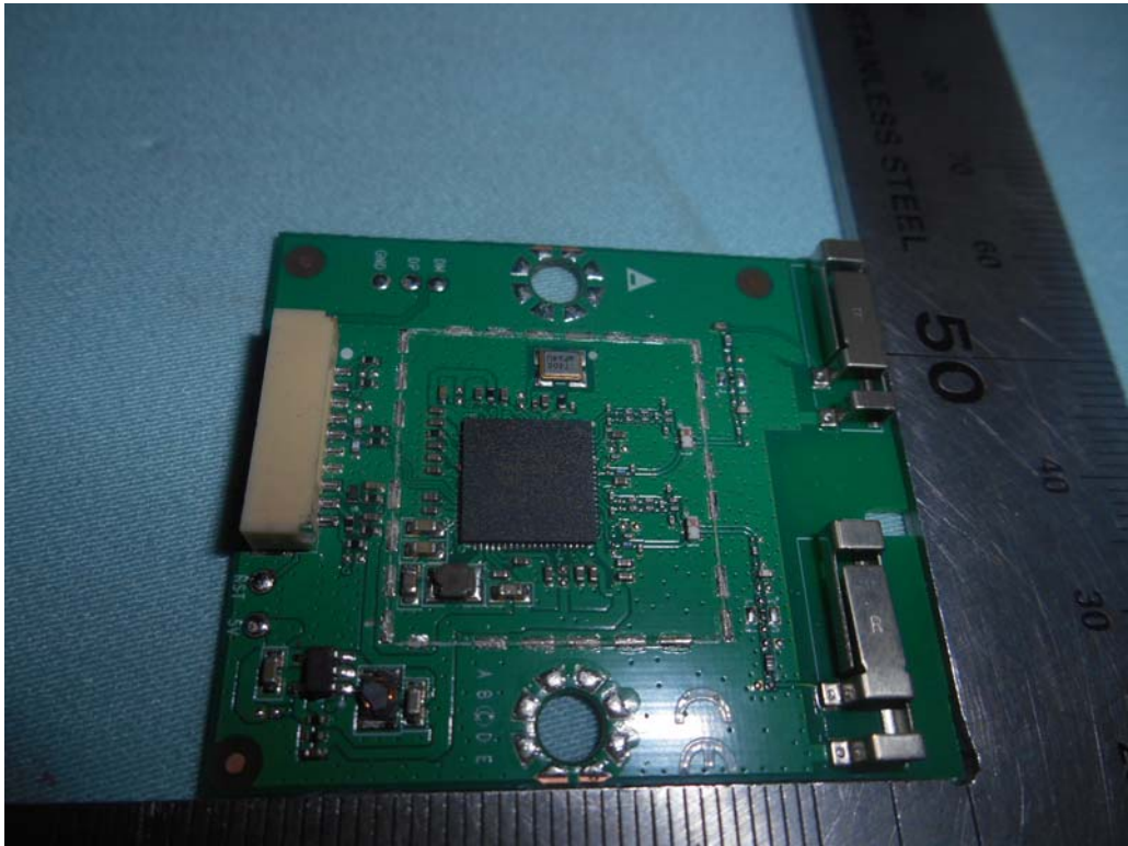
FIGURE 11 LED LCD TV (M/N: LC-65P7000U) RF BOARD COVER REMOVED
