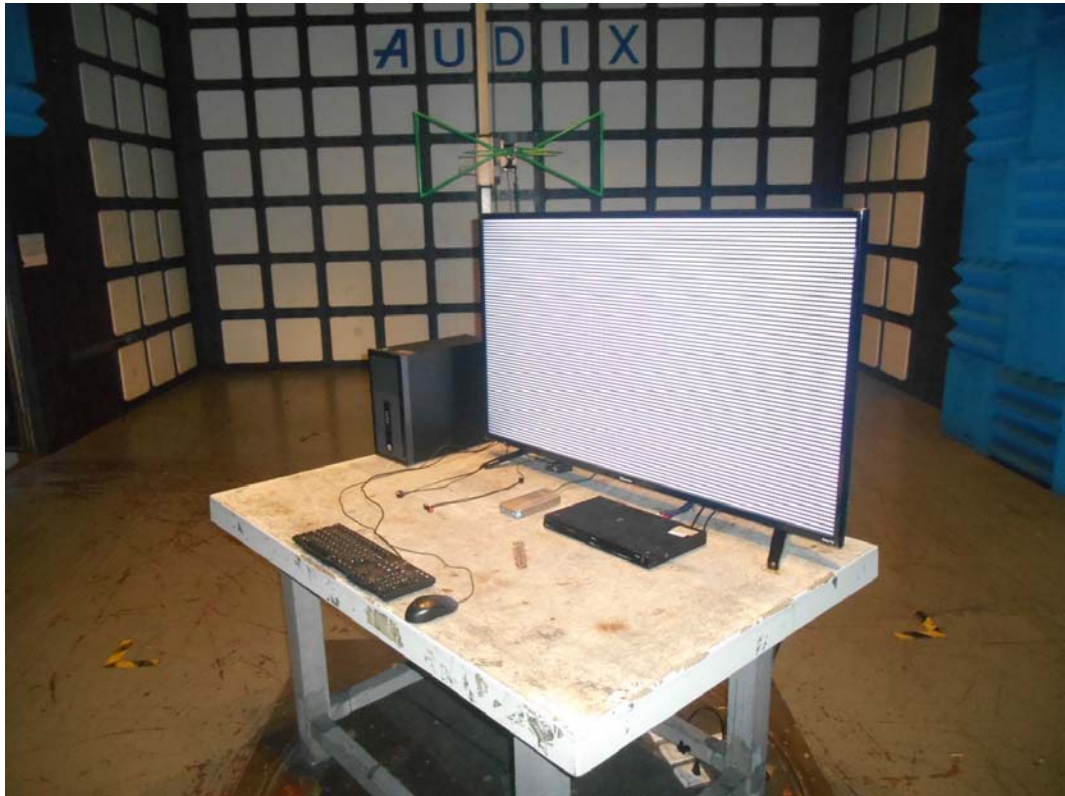
SETUP WITH MAXIMUM DETECTED EMISSION AT HORIZONTAL POLARIZATION (TEST MODE: HDMI 3840*2160@60Hz & 1KHz PLAYING)
