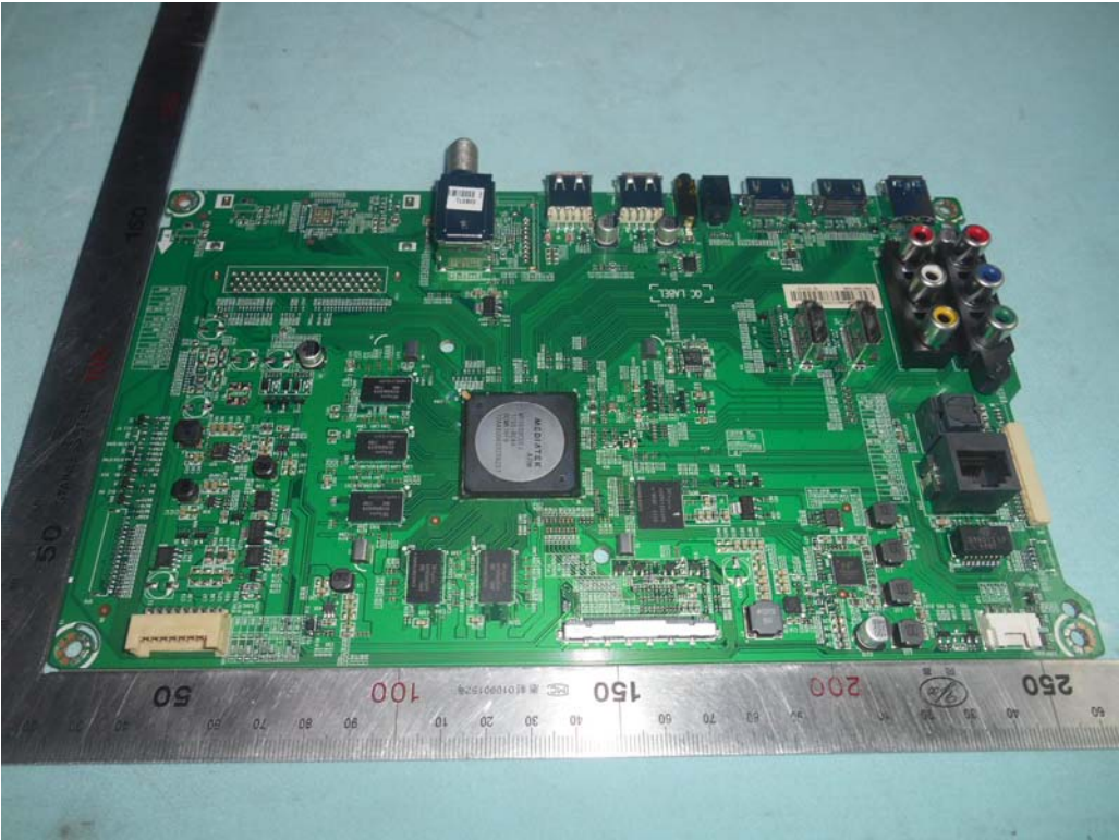
FIGURE 2 LED LCD TV (M/N: 50H6D) MAIN BOARD (COMPONENT SIDE)
