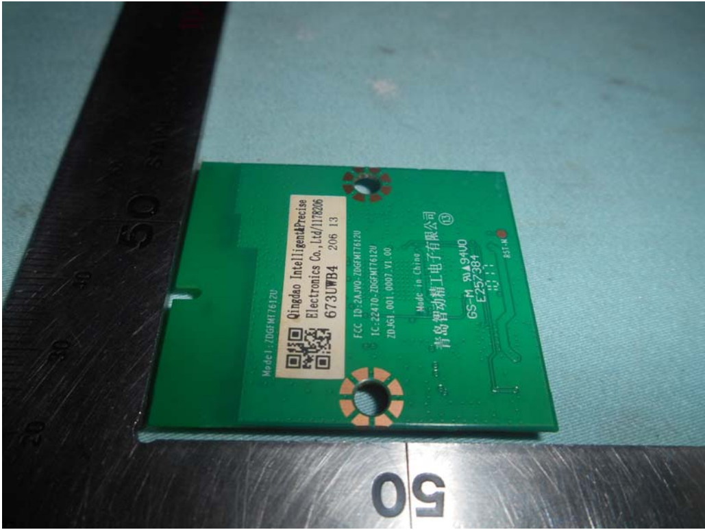
FIGURE 10 LED LCD TV (M/N: 50H6D) RF BOARD (SOLDERED SIDE)
