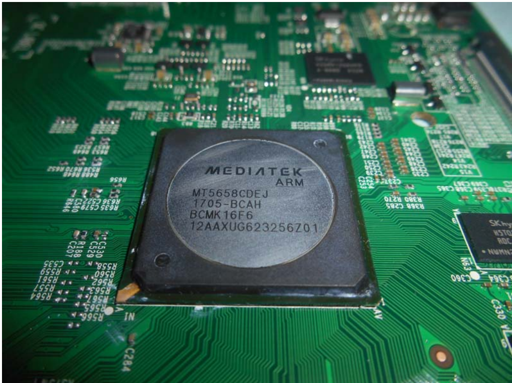
FIGURE 4 LED LCD TV (M/N: 50H6D) CHIP AND CRYSTAL ON MAIN BOARD
