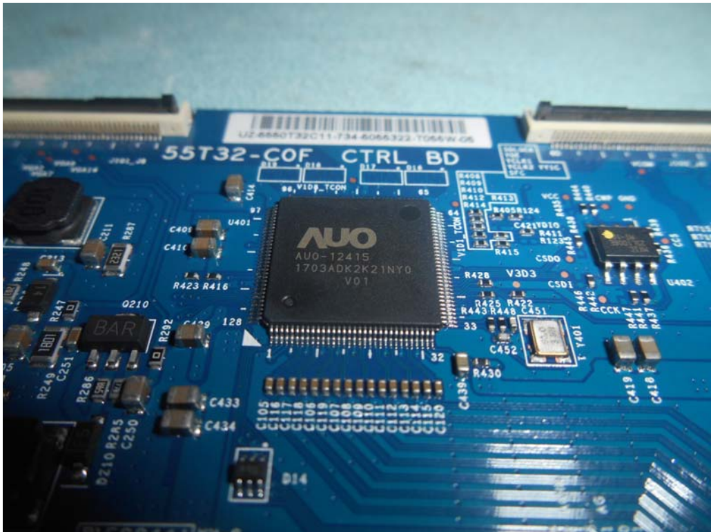
FIGURE 8 LED LCD TV (M/N: 50H6D) CHIP AND CRYSTAL ON PANEL BOARD
