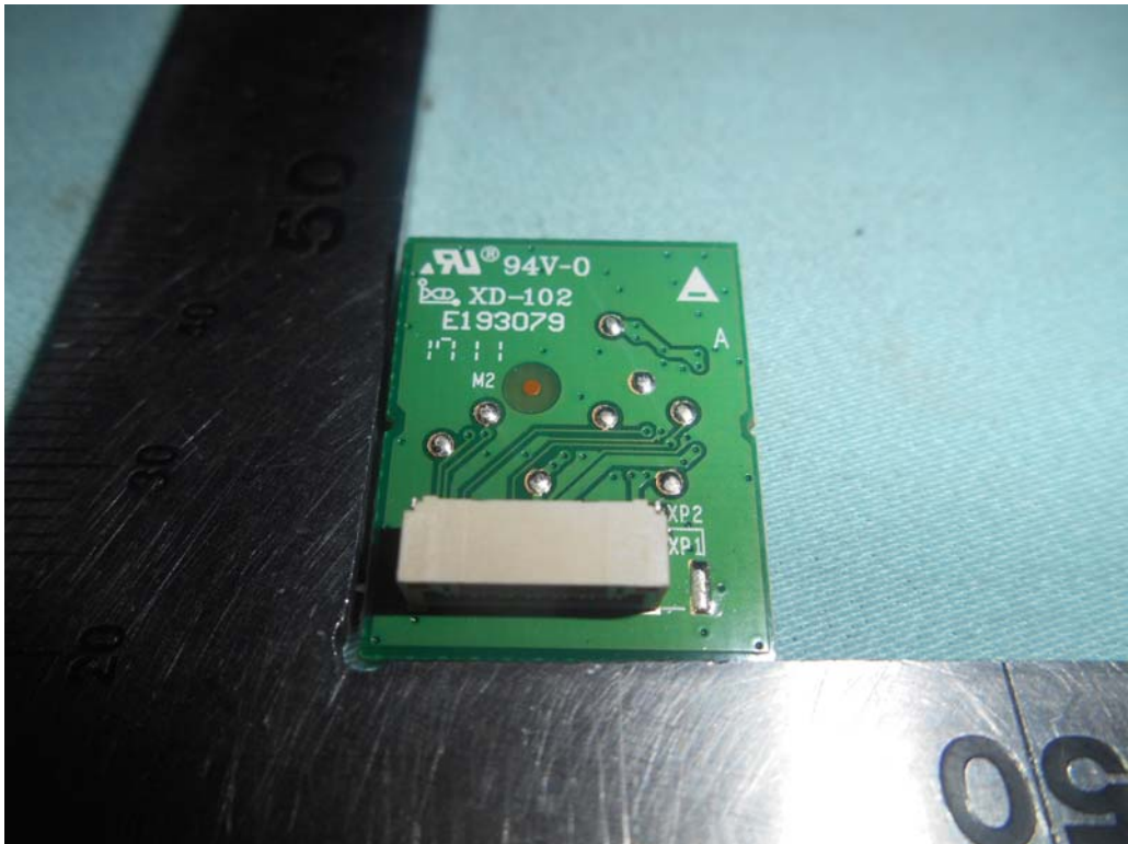
FIGURE 16 LED LCD TV (M/N: 50H6D) IR BOARD (SOLDERED SIDE)
