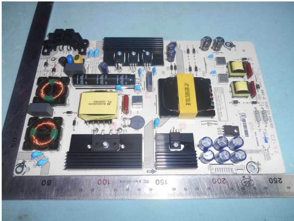
FIGURE 17 LED LCD TV (M/N: 50H6D) POWER BOARD (COMPONENT SIDE)
