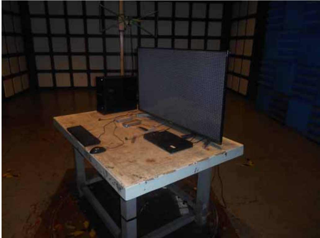
SETUP WITH MAXIMUM DETECTED EMISSION AT HORIZONTAL POLARIZATION (TEST MODE: HDMI2 1920*1080@60Hz & 1KHz PLAYING)
