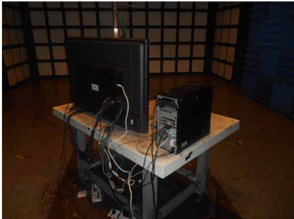
SETUP WITH MAXIMUM DETECTED EMISSION AT VERTICAL POLARIZATION (TEST MODE: HDMI2 1920*1080@60Hz & 1KHz PLAYING)
