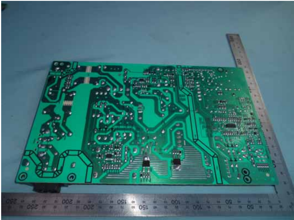
FIGURE 4 LED LCD TV (M/N: LC-50P5000U) POWER BOARD (SOLDERED SIDE)
