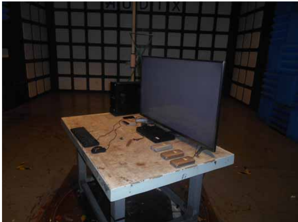
SETUP WITH MAXIMUM DETECTED EMISSION AT VERTICAL POLARIZATION (TEST MODE: HDMI3 3840*2160@30Hz & 1KHz PLAYING)
