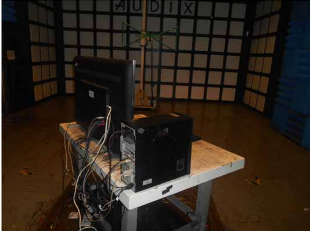
SETUP WITH MAXIMUM DETECTED EMISSION AT HORIZONTAL POLARIZATION (TEST MODE: HDMI3 3840*2160@30Hz & 1KHz PLAYING)
