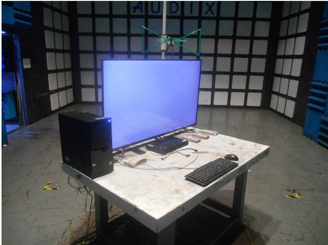
SETUP WITH MAXIMUM DETECTED EMISSION AT HORIZONTAL POLARIZATION (TEST MODE: HDMI4 3840*2160@60Hz & 1kHz PLAYING)
