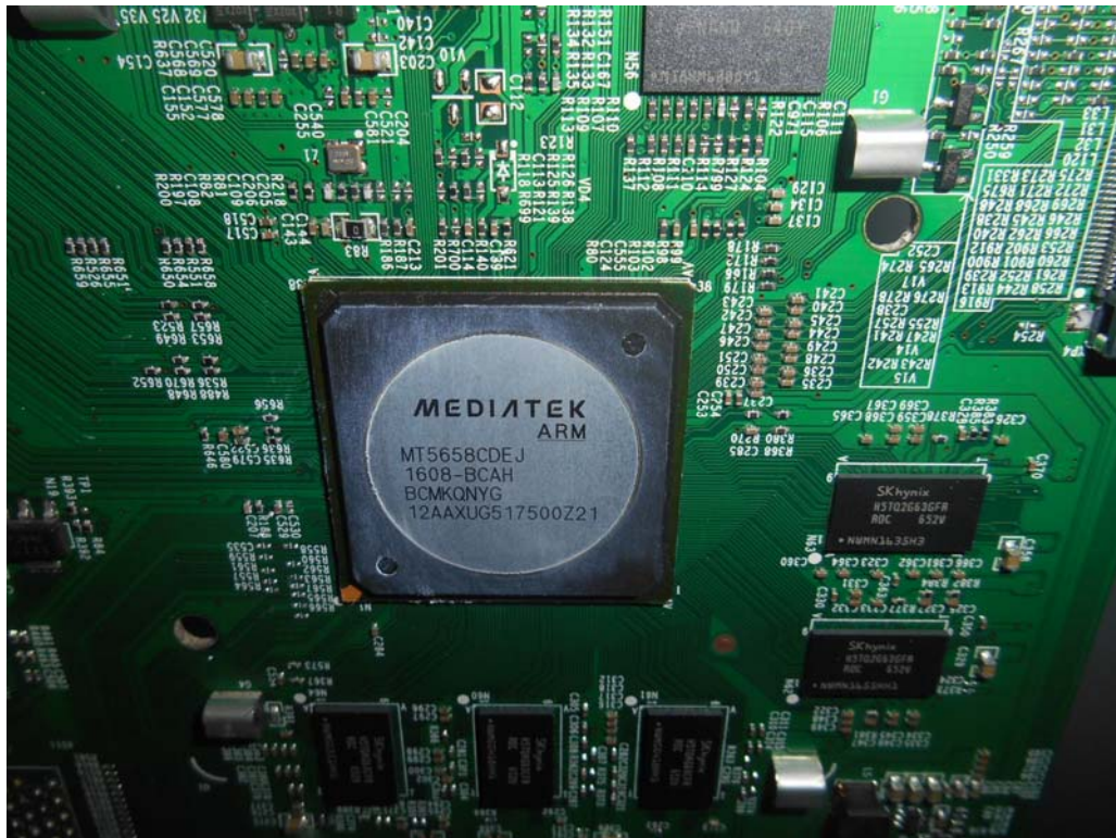
FIGURE 7 LED LCD TV (M/N: 65H8C) CHIP & CRYSTAL ON MAIN BOARD
