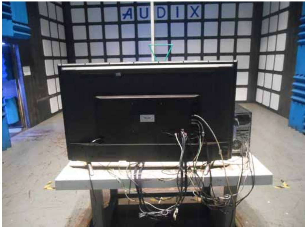
SETUP WITH MAXIMUM DETECTED EMISSION AT VERTICAL POLARIZATION (TEST MODE: HDMI3 3840*2160@60Hz & 1KHz PLAYING)
