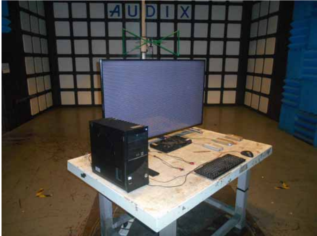
SETUP WITH MAXIMUM DETECTED EMISSION AT HORIZONTAL POLARIZATION (TEST MODE: HDMI3 3840*2160@60Hz & 1KHz PLAYING)
