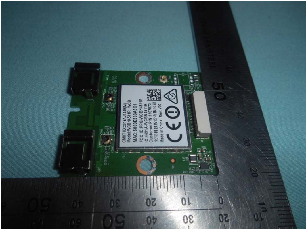
FIGURE 14 LED LCD TV (M/N: 55H9D) RF BOARD (COMPONENT SIDE)
