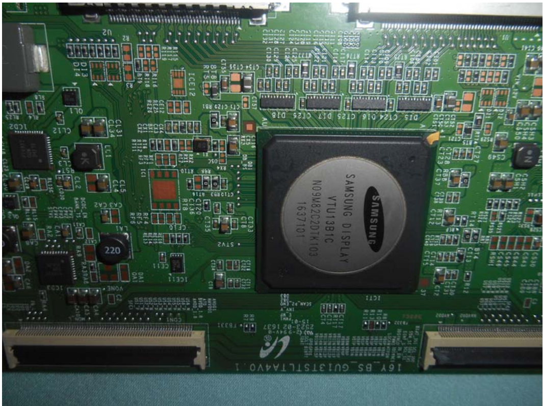
FIGURE 20 LED LCD TV(M/N: 55H9D) CHIP AND CRYSTAL ON PANEL BOARD
