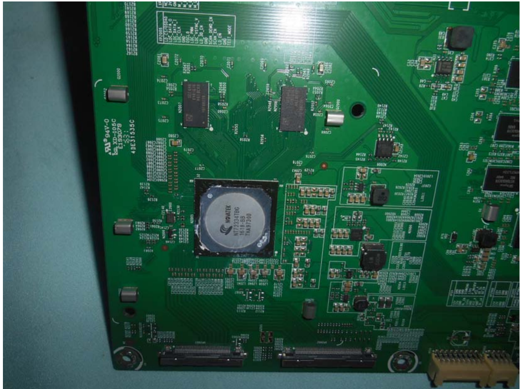
FIGURE 9 LED LCD TV(M/N: 55H9D) CHIP#1 AND CRYSTAL#1 ON MAIN BOARD
