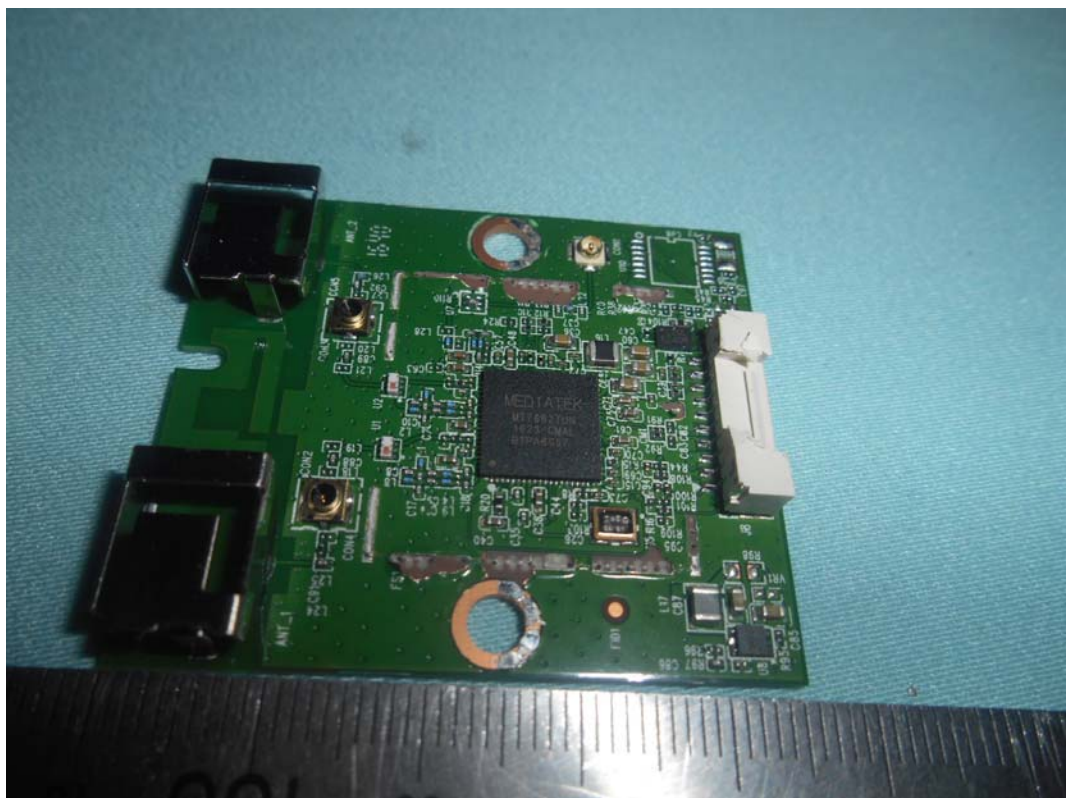
FIGURE 17 LED LCD TV (M/N: 55H9D) CHIP AND CRYSTAL ON RF BOARD
