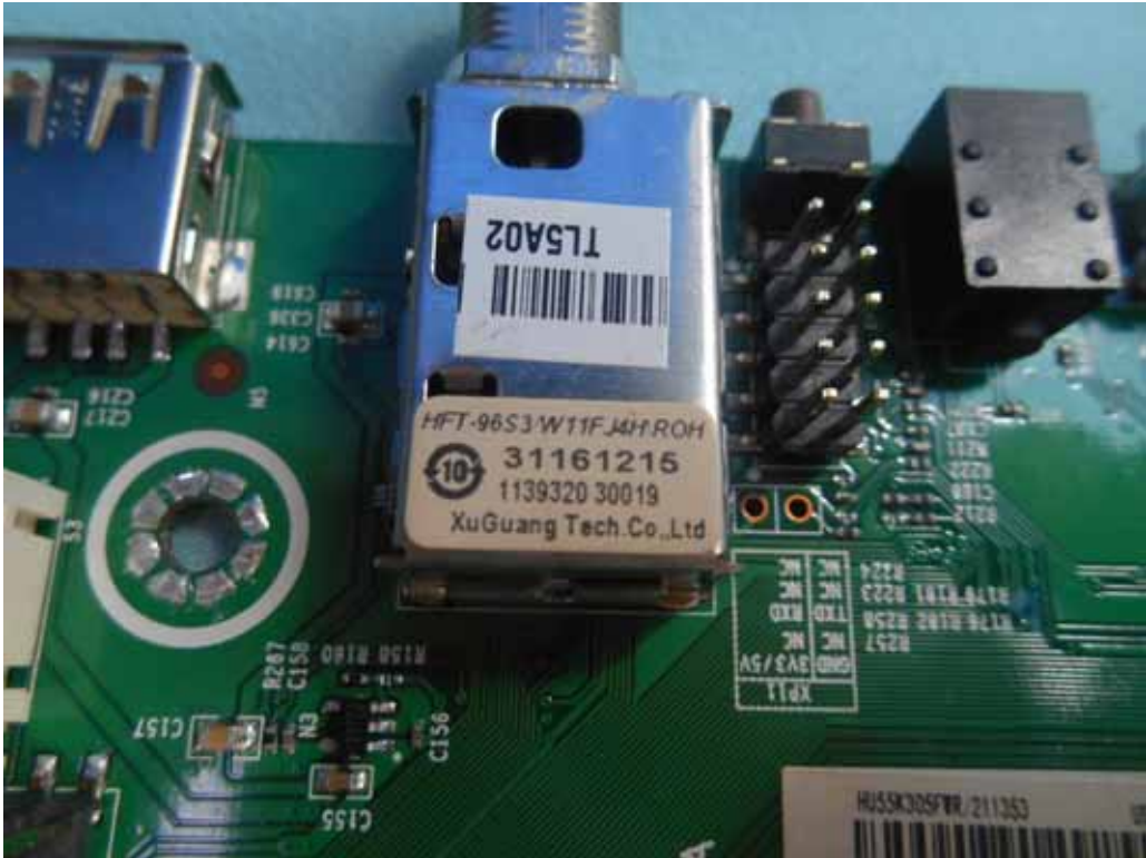
FIGURE 6 LED LCD TV (M/N: 55H4D) TUNER
