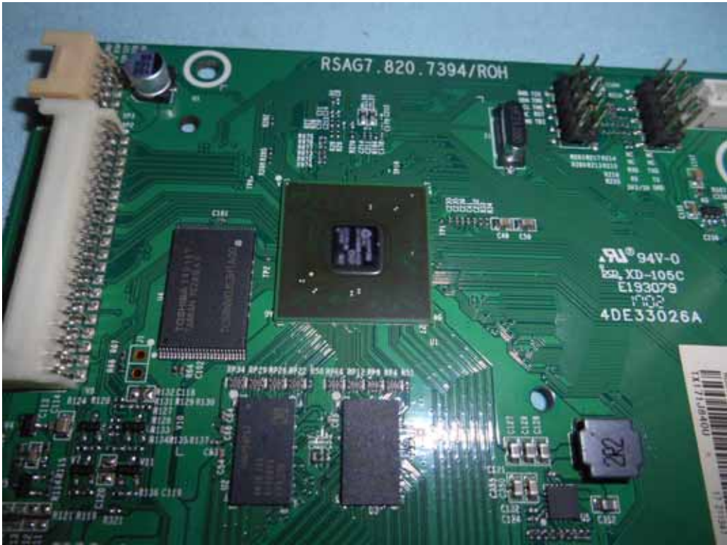
FIGURE 5 LED LCD TV (M/N: 55H4D) CHIP & CRYSTAL ON MAIN BOARD
