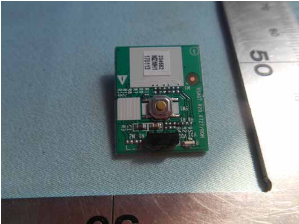
FIGURE 14 LED LCD TV (M/N: 55H4D) KEY BOARD (COMPONENT SIDE)
