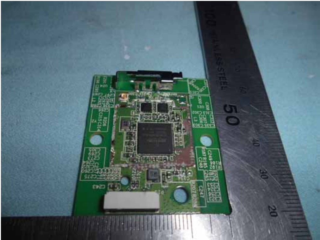
FIGURE 7 LED LCD TV (M/N: 55H4D) RF BOARD (COMPONENT SIDE)
