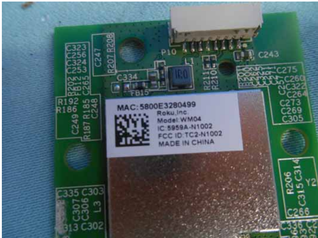
FIGURE 9 LED LCD TV (M/N: 55H4D) RF LABEL
