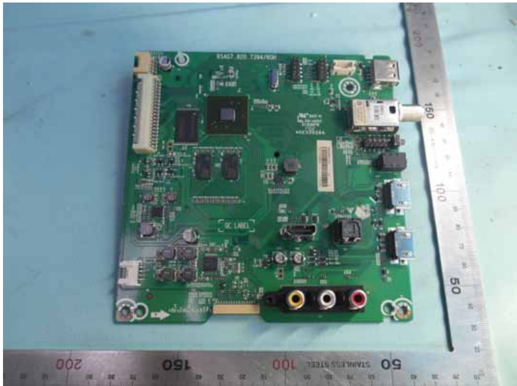
FIGURE 3 LED LCD TV (M/N: 55H4D) MAIN BOARD (COMPONENT SIDE)
