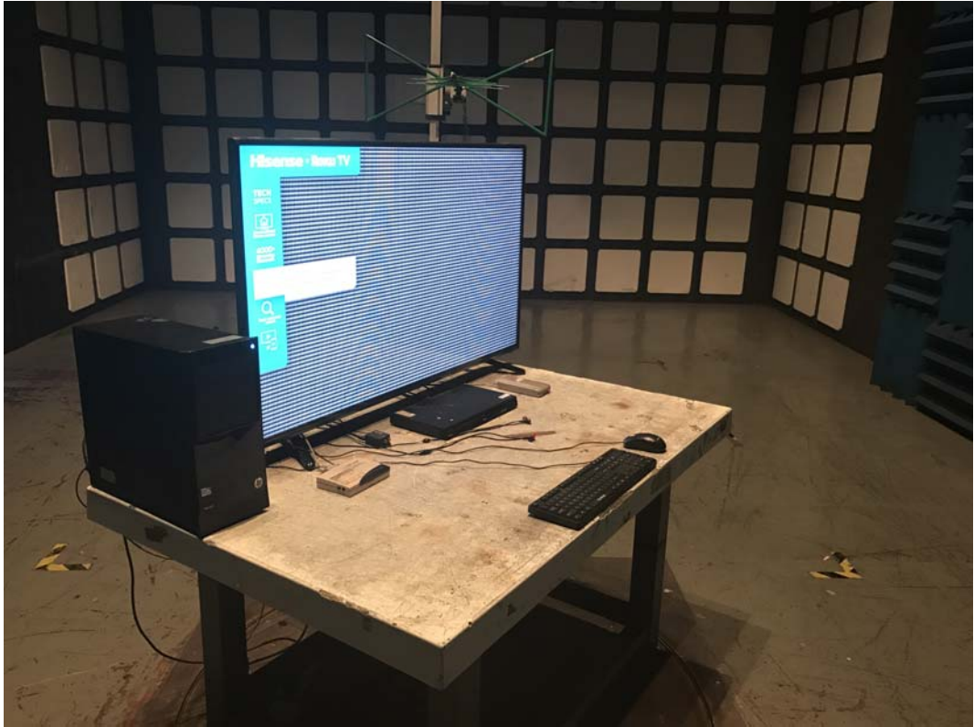
SETUP WITH MAXIMUM DETECTED EMISSION AT HORIZONTAL POLARIZATION (TEST MODE: HDMI1 1920*1080@60Hz & 1kHz PLAYING)
