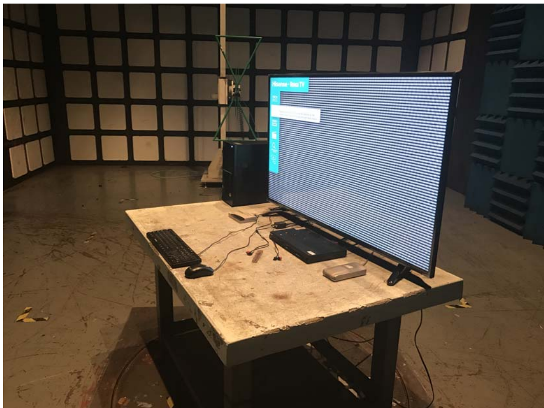
SETUP WITH MAXIMUM DETECTED EMISSION AT VERTICAL POLARIZATION (TEST MODE: HDMI1 1920*1080@60Hz & 1kHz PLAYING)
