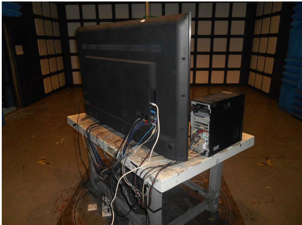
SETUP WITH MAXIMUM DETECTED EMISSION AT VERTICAL POLARIZATION (TEST MODE: HDMI 3840*2160@60Hz & 1kHz PLAYING)
