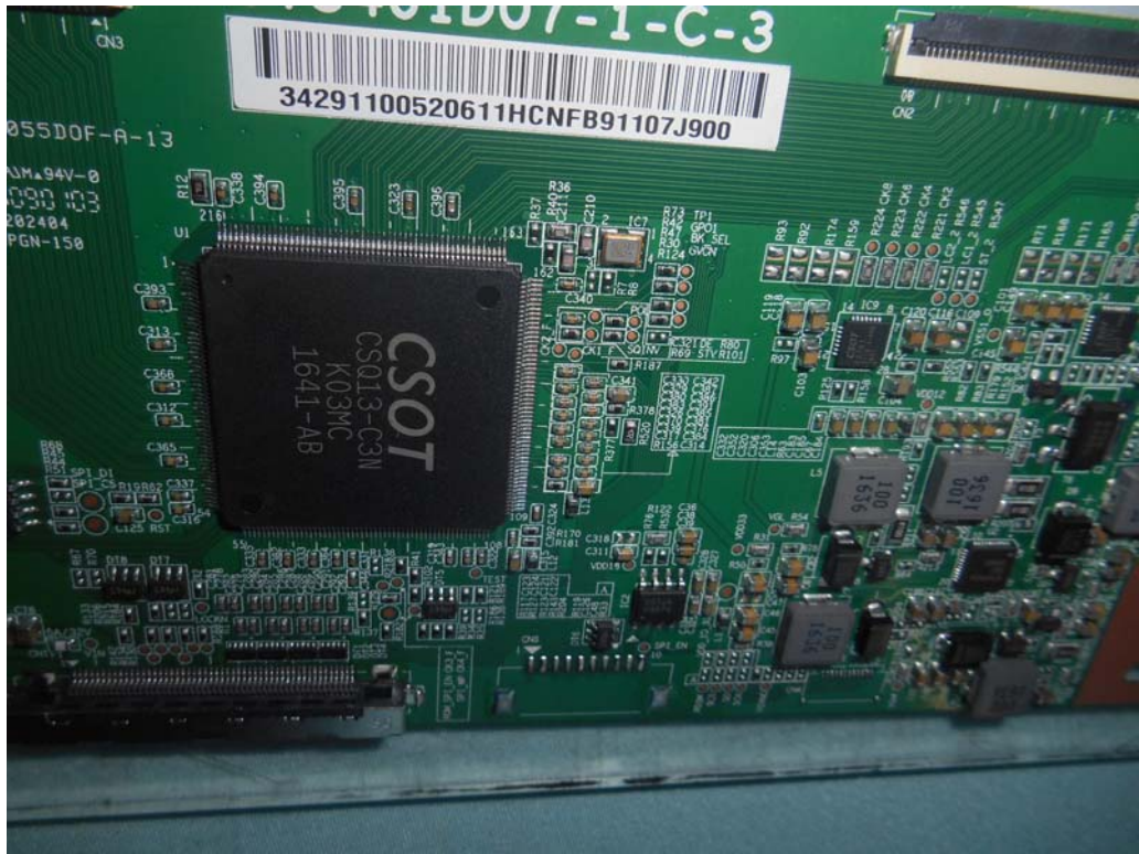
FIGURE 12 LED LCD TV (M/N: HU55N3000UW) CHIP & CRYSTAL ON PANEL BOARD
