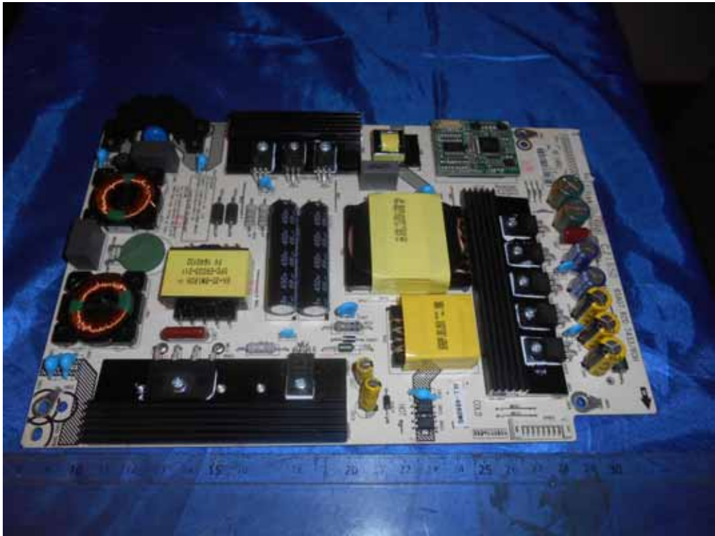
FIGURE 7 LED LCD TV (M/N: LC-55P8000U) POWER BOARD (COMPONENT SIDE)
