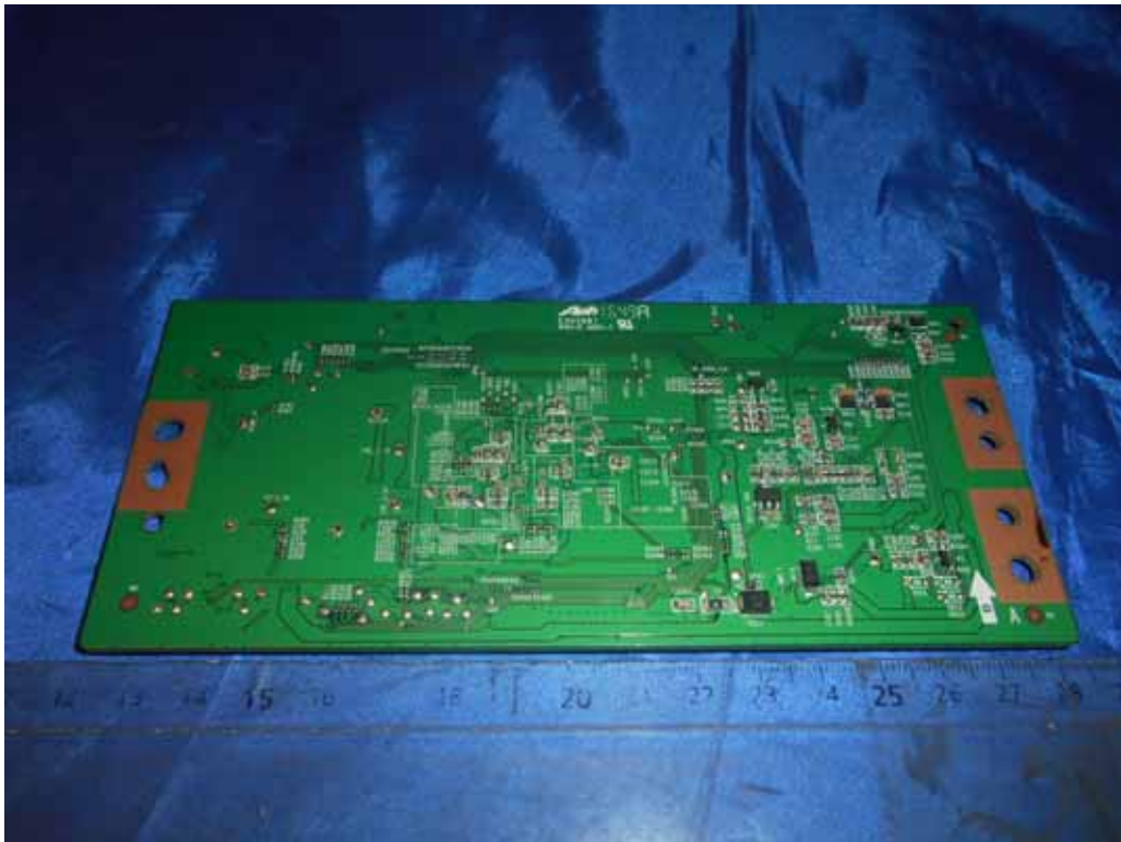
FIGURE 10 LED LCD TV (M/N: LC-55P8000U) PANEL BOARD (SOLDERED SIDE)
