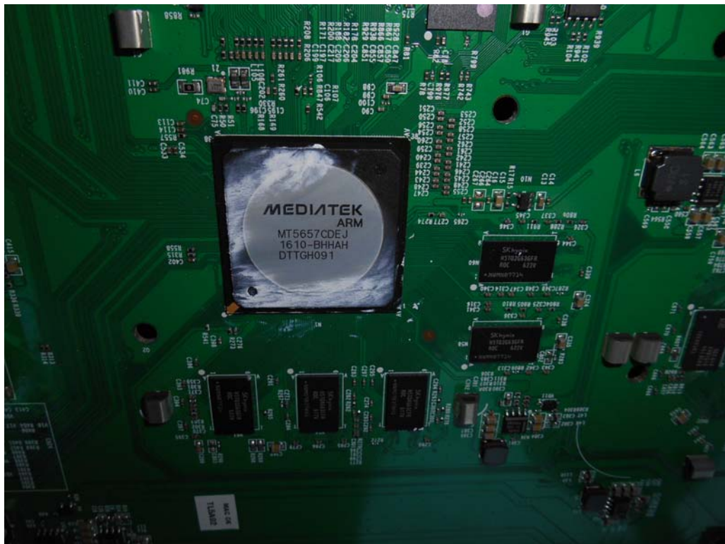
FIGURE 8 LED LCD TV (M/N: LC-75U) CHIP AND CRYSTAL#1 ON MAIN BOARD
