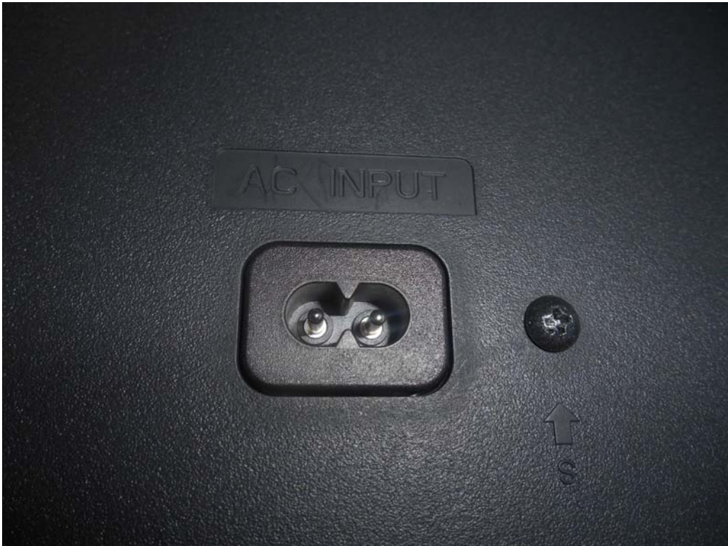
FIGURE 3 LED LCD TV (M/N: LC-75U) AC PORT
