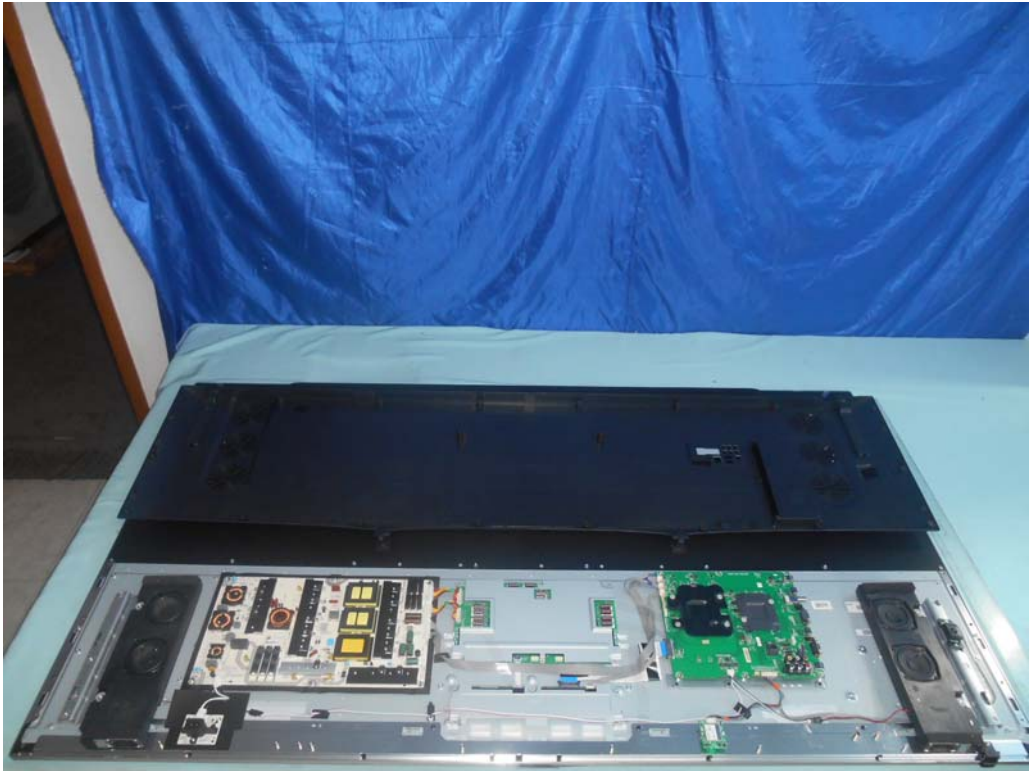
FIGURE 6 LED LCD TV (M/N: LC-75U) COVER REMOVED
