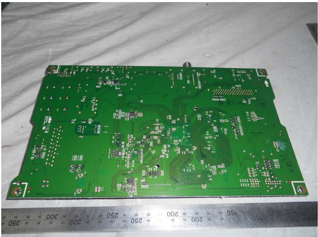
FIGURE 4 LED LCD TV (M/N: LC-55N7000U) MAIN BOARD (SOLDERED SIDE)
