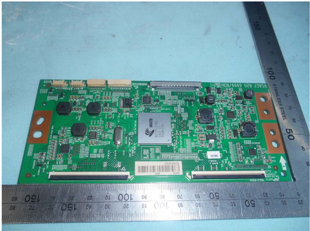
FIGURE 12 LED LCD TV (M/N: LC-55U) PANEL BOARD (COMPONENT SIDE)
