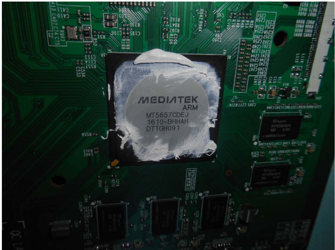
FIGURE 7 LED LCD TV (M/N: LC-55U) CHIP AND CRYSTAL ON MAIN BOARD
