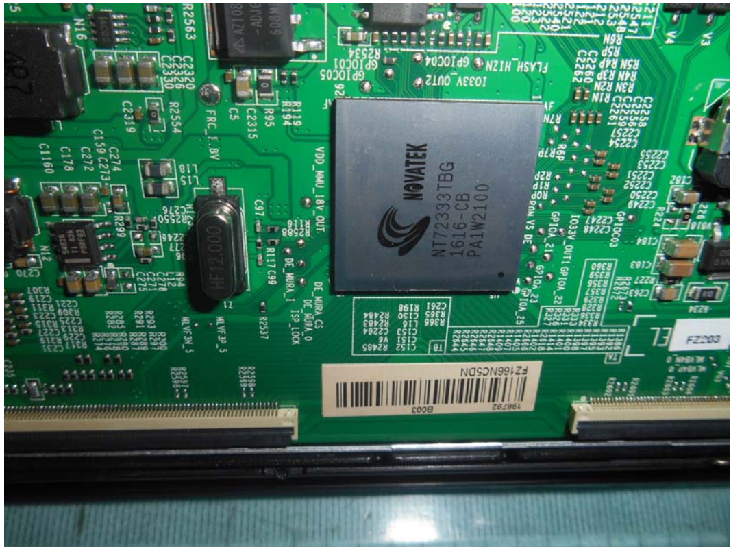
FIGURE 14 LED LCD TV (M/N: LC-55U) CHIP ON PANEL BOARD
