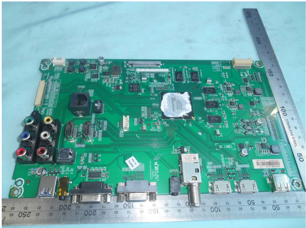
FIGURE 5 LED LCD TV (M/N: LC-55U) MAIN BOARD (COMPONENT SIDE)
