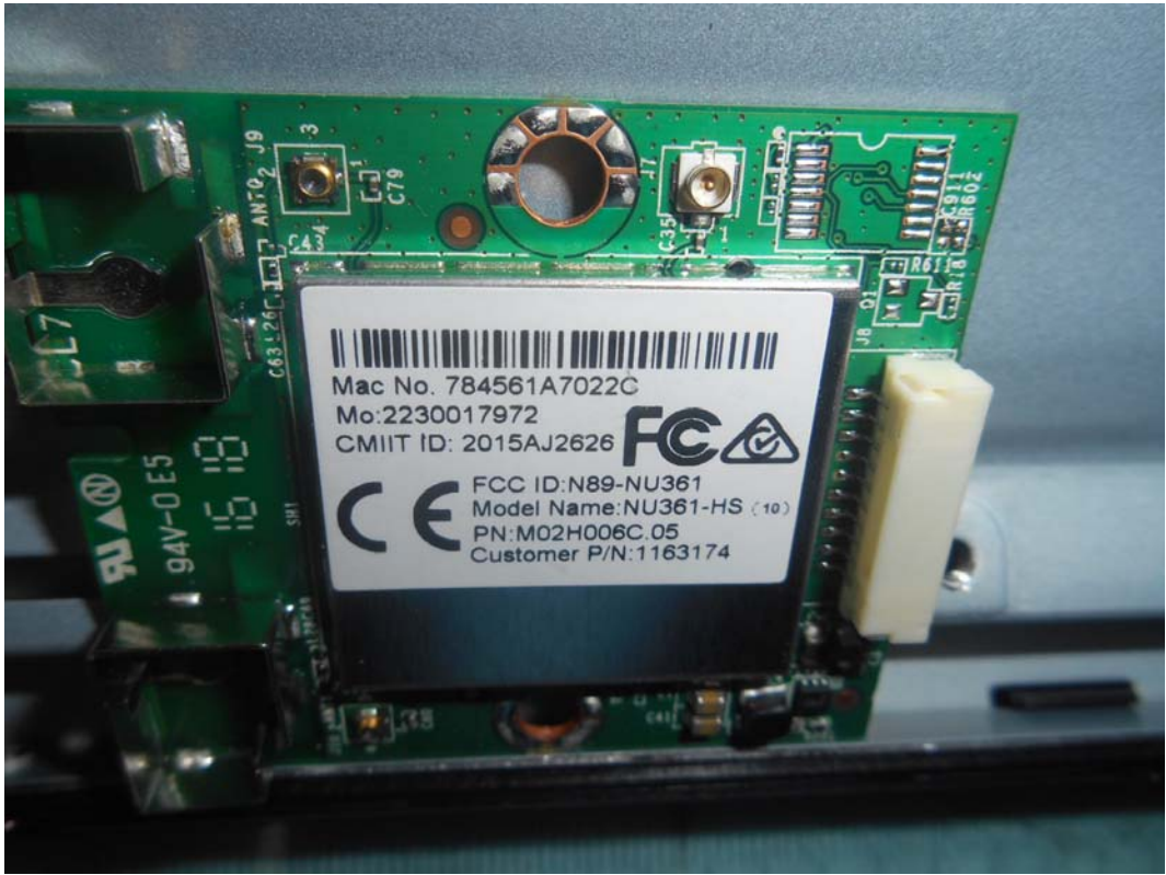
FIGURE 21 LED LCD TV (M/N: LC-55U) RF BOARD LABEL
