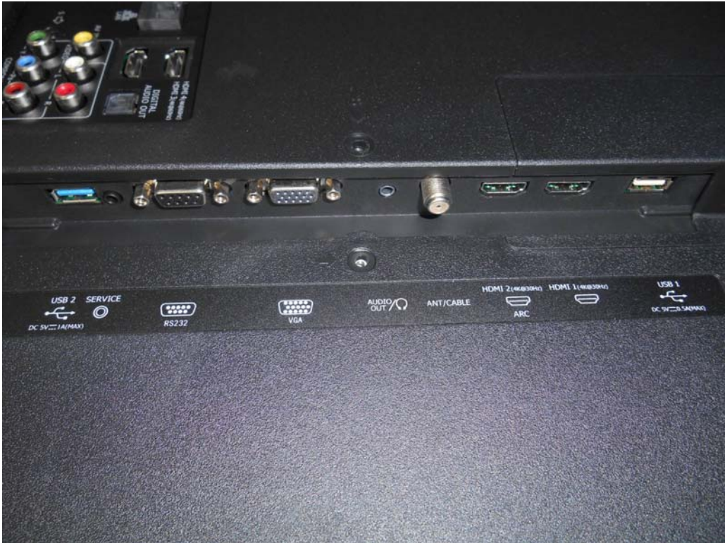
FIGURE 4 LED LCD TV (M/N: 65U1600) PORTS #2
