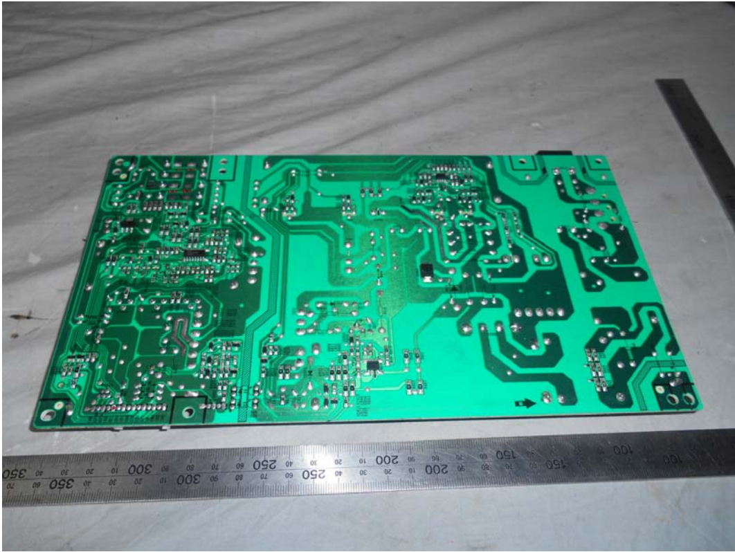
FIGURE 18 LED LCD TV (M/N: LC-55N7000U) POWER BOARD (SOLDERED SIDE)
