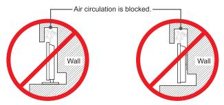
Inadequate air circulation can cause the TV to overheat.
