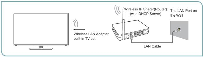
PROSCAN's built-in Wireless LAN Adapter supports the IEEE 802.11 b/g/n communication protocols. PROSCAN recommends using IEEE 802.11n router. When you play the video over a IEEE 802.11b/g connection, the video may not play smoothly.
