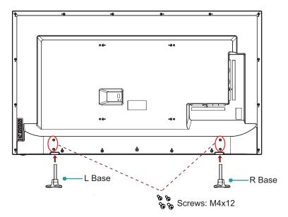
Plug the Left base and the Right base separately in the mounting holes at the bottom of the machine, and then use two M4x12 screws to fix the base and the whole machine together.
