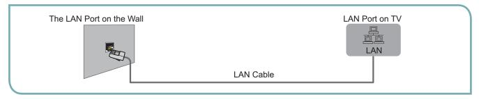
If you have a Dynamic Network, you should use an ADSL modem or router that supports Dynamic Host Configuration Protocol (DHCP). Modems and routers that support DHCP automatically provide the IP address, subnet mask, gateway, and DNS, so you don't have to enter them manually. Most home networks are Dynamic Networks.
