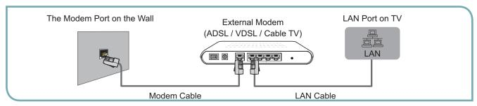
You can attach your TV to your LAN by connecting the LAN port on the back of your TV to an IP Sharer which is connected
