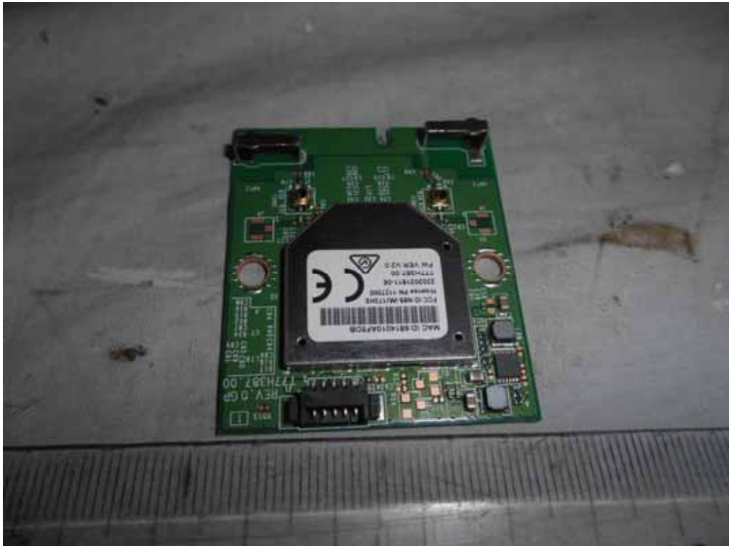
FIGURE 9 LED LCD TV (M/N: PLDED6079-SM) RF BOARD (COMPONENT SIDE)
