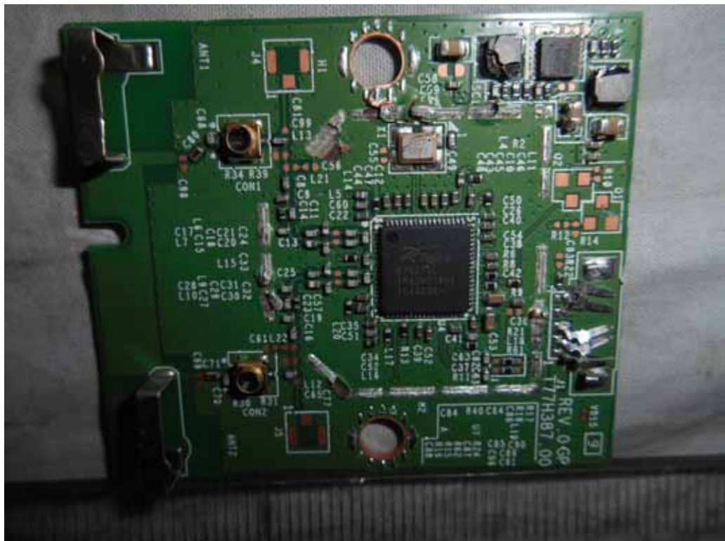
FIGURE 12 LED LCD TV (M/N: PLDED6079-SM) RF BOARD COVER REMOVED
