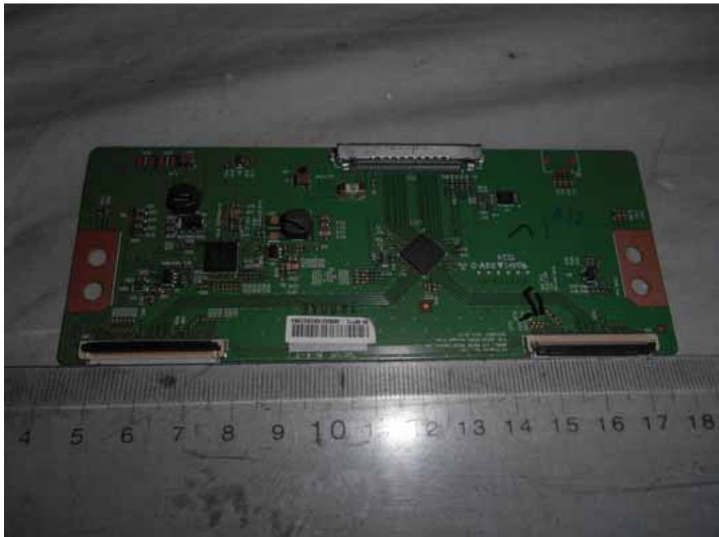
FIGURE 13 LED LCD TV (M/N: PLDED6079-SM) PANEL BOARD (COMPONENT SIDE)
