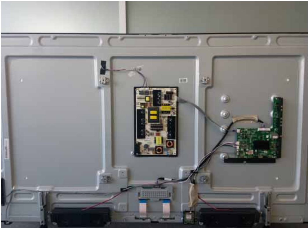
FIGURE 1 LED LCD TV (M/N: PLDED6079-SM) COVER REMOVED
