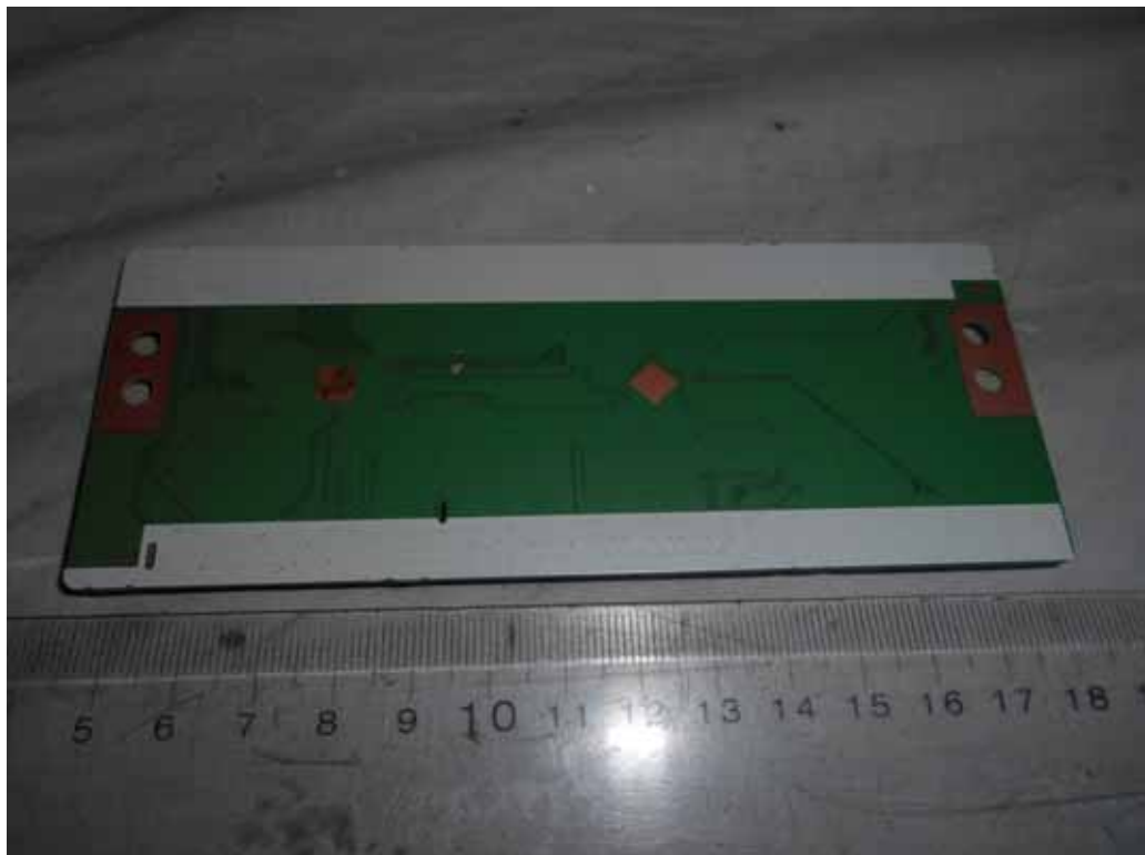
FIGURE 14 LED LCD TV (M/N: PLDED6079-SM) PANEL BOARD (SOLDERED SIDE)
