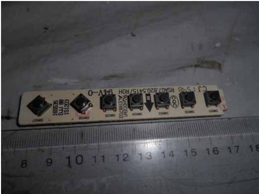
FIGURE 18 LED LCD TV (M/N: PLDED6079-SM) KEY BOARD (COMPONENT SIDE)
