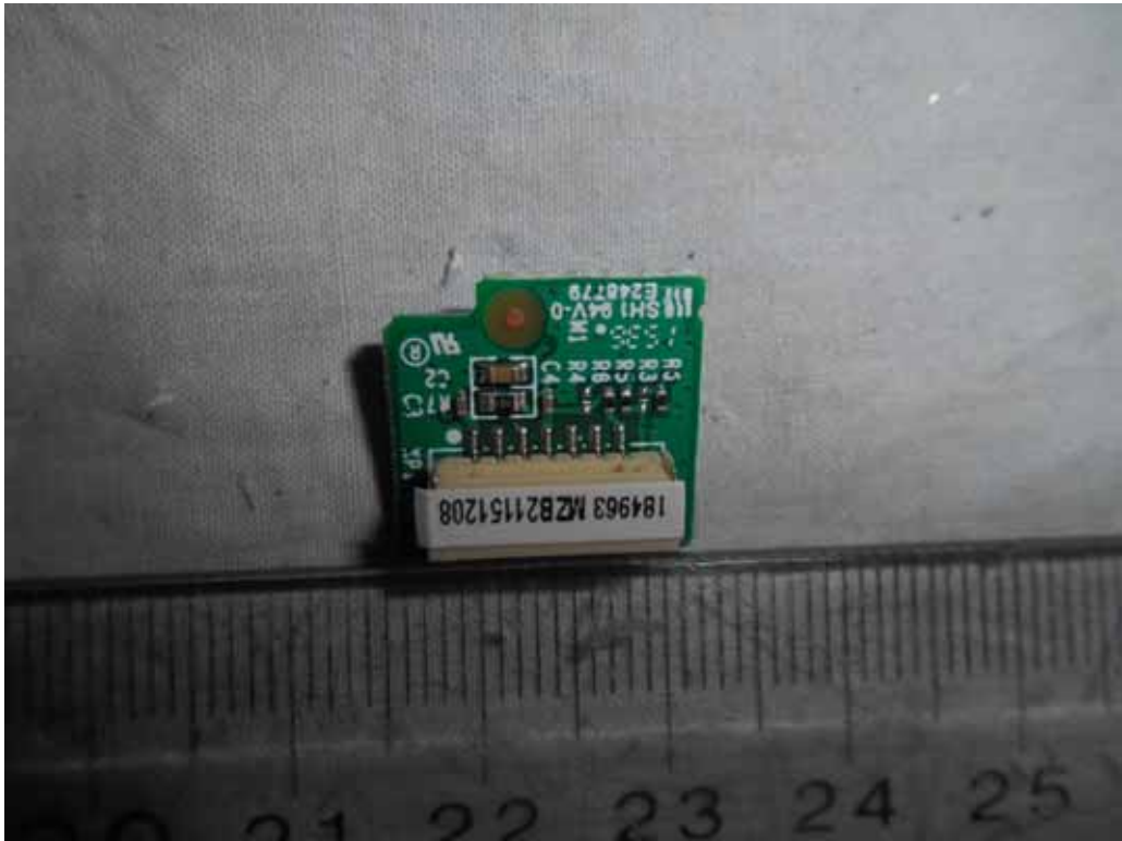
FIGURE 21 LED LCD TV (M/N: PLDED6079-SM) IR BOARD (SOLDERED SIDE)
