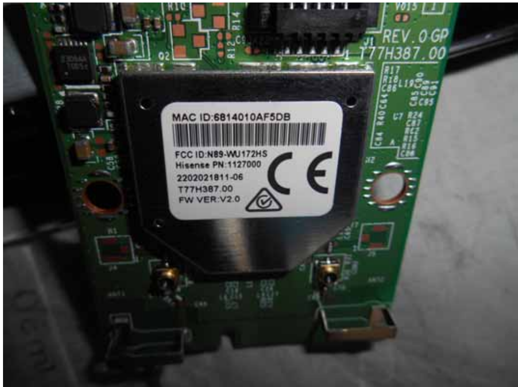
FIGURE 11 LED LCD TV (M/N: PLDED6079-SM) RF BOARD LABEL
