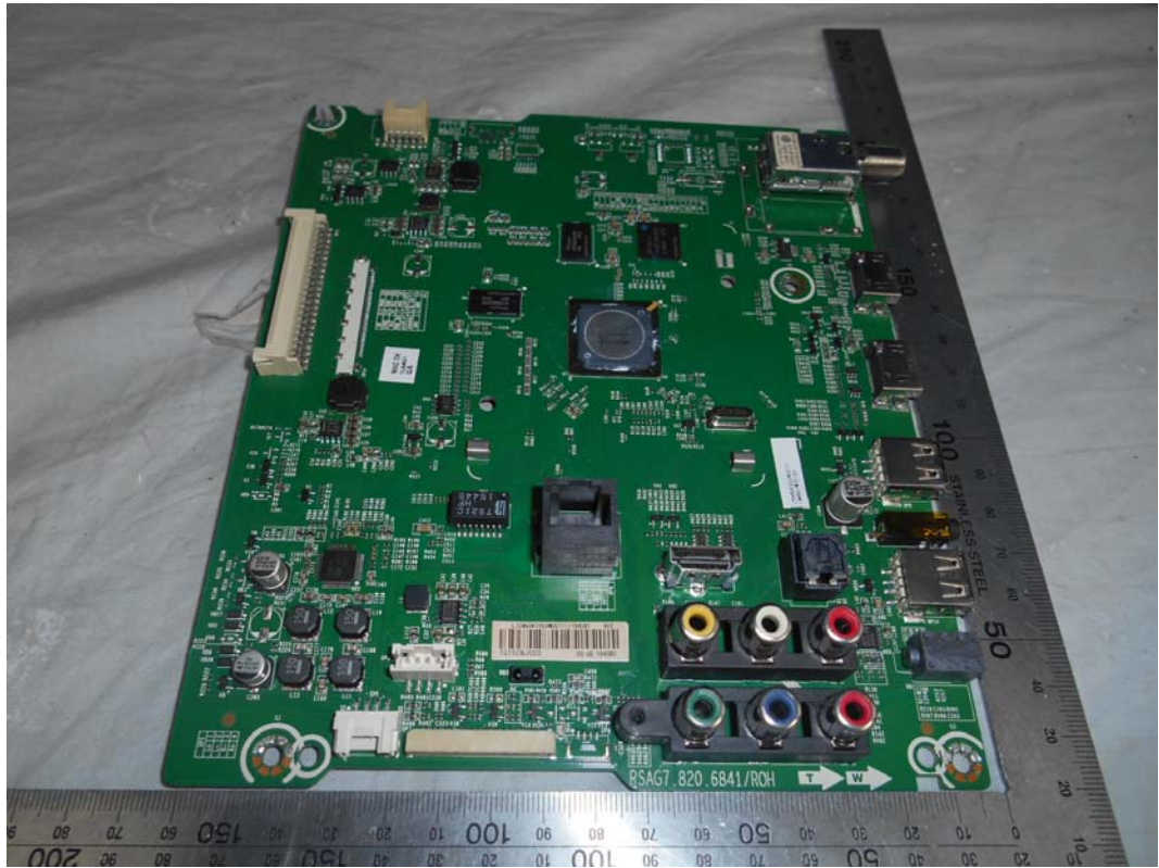
FIGURE 3 LED LCD TV (M/N: 50K2203W) MAIN BOARD (COMPONENT SIDE)
