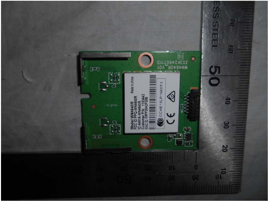
FIGURE 13 LED LCD TV (M/N: 50K2203W) RF BOARD (COMPONENT SIDE)
