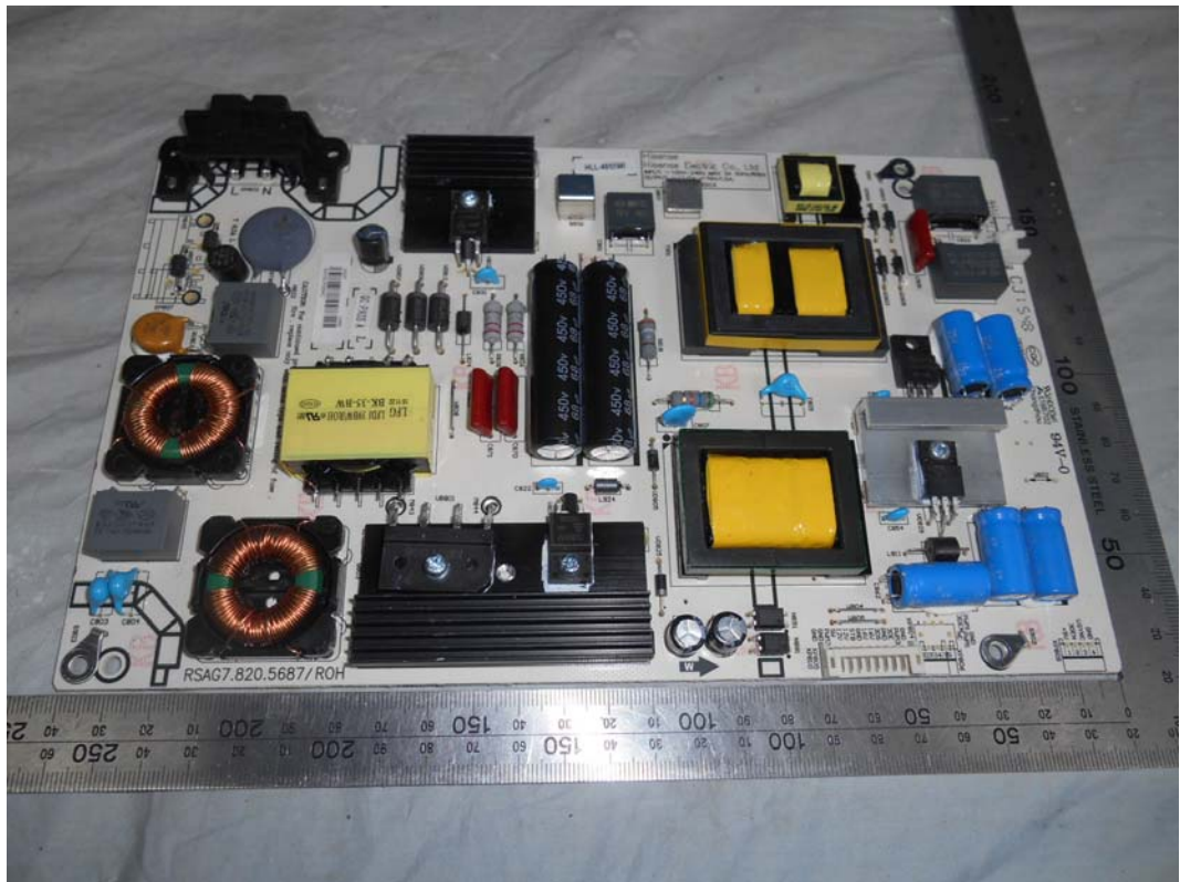
FIGURE 17 LED LCD TV (M/N: 50K2203W) POWER BOARD (COMPONENT SIDE)
