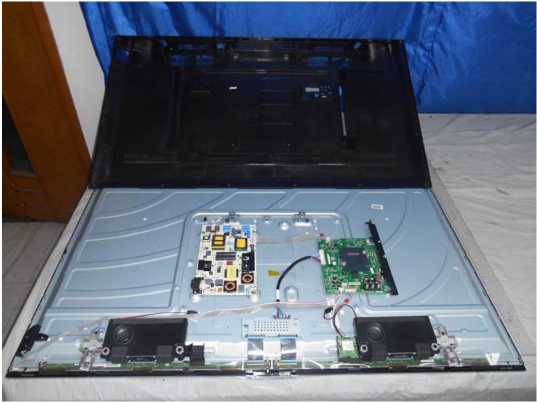
FIGURE 1 LED LCD TV (M/N: 50K2203W) COVER REMOVED
