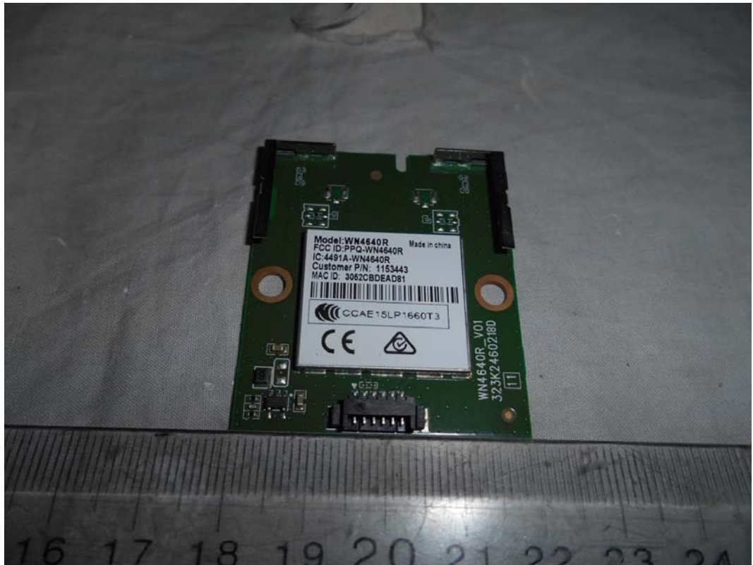
FIGURE 10 LED LCD TV (M/N: LC-60N5100U) RF BOARD (COMPONENT SIDE)
