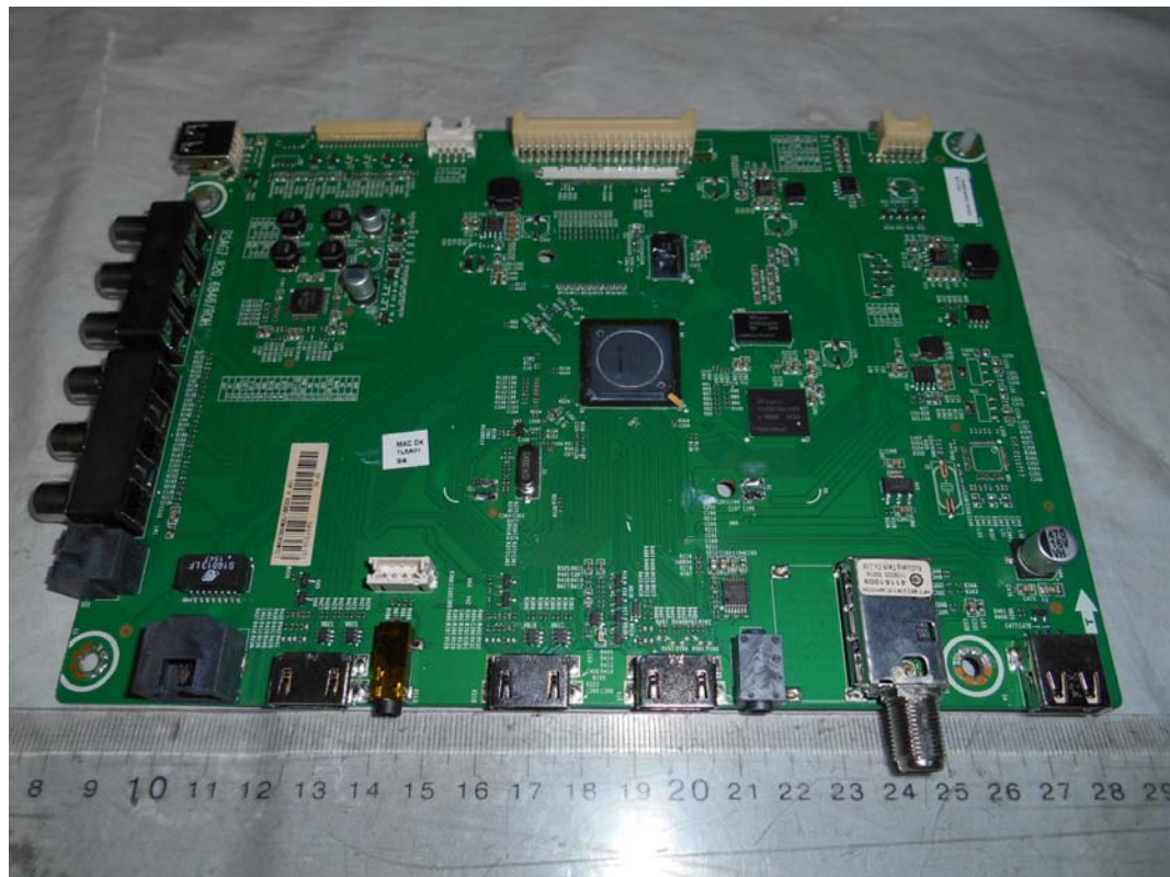
FIGURE 3 LED LCD TV (M/N: LC-60N5100U) MAIN BOARD (COMPONENT SIDE)
