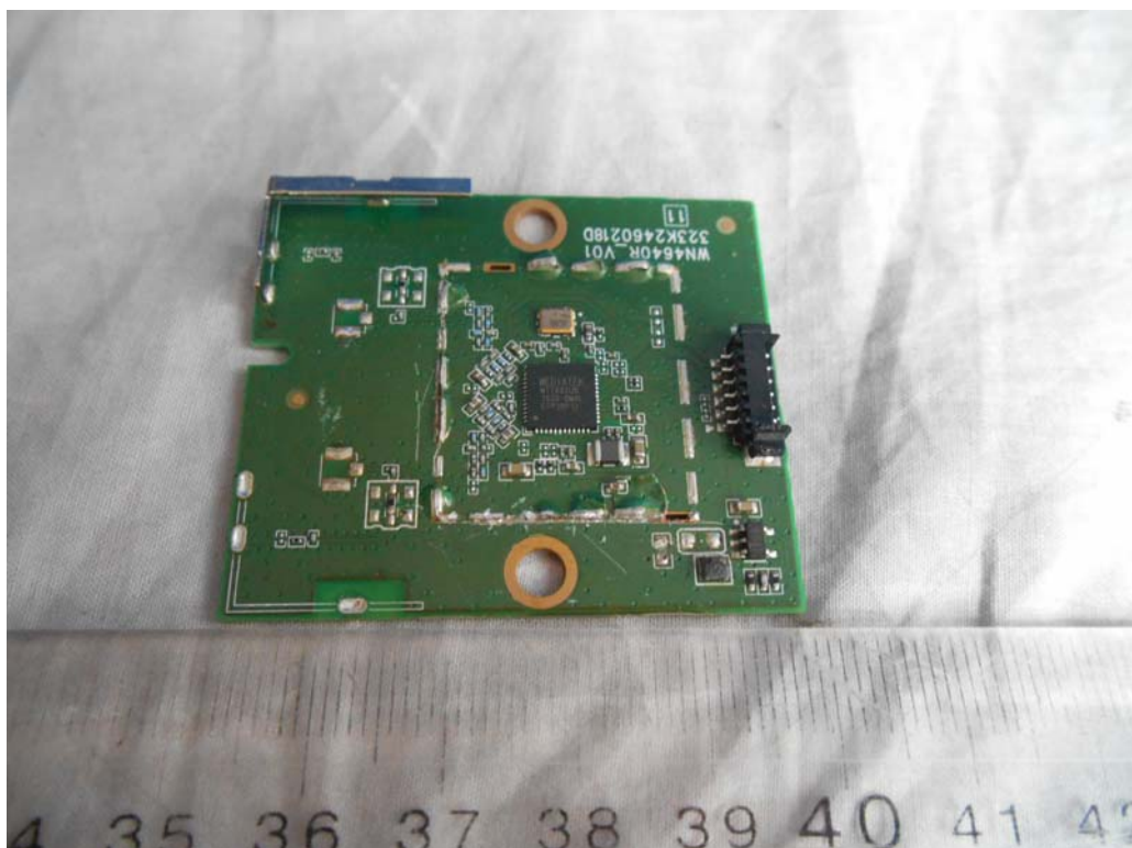
FIGURE 13 LED LCD TV (M/N: LC-60N5100U) RF BOARD COVER REMOVED
