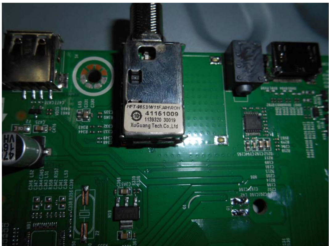
FIGURE 6 LED LCD TV (M/N: LC-60N5100U) TUNER
