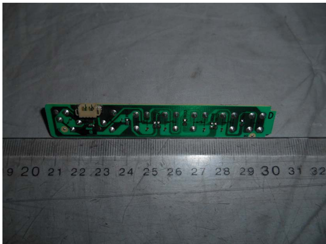
FIGURE 17 LED LCD TV (M/N: LC-60N5100U) KEY BOARD (SOLDERED SIDE)
