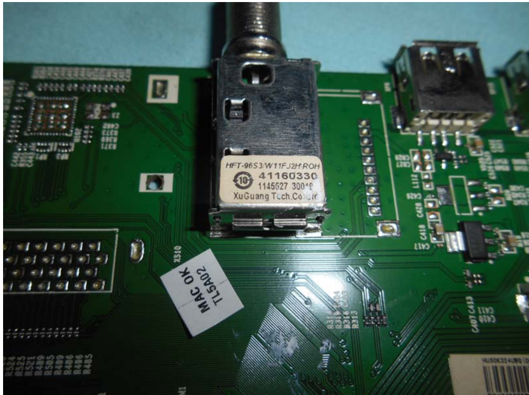
FIGURE 6 LED LCD TV (M/N: LC-50N6000U) TUNER
