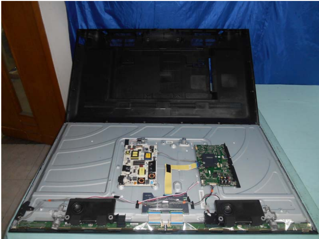
FIGURE 1 LED LCD TV (M/N: LC-50N6000U) COVER REMOVED
