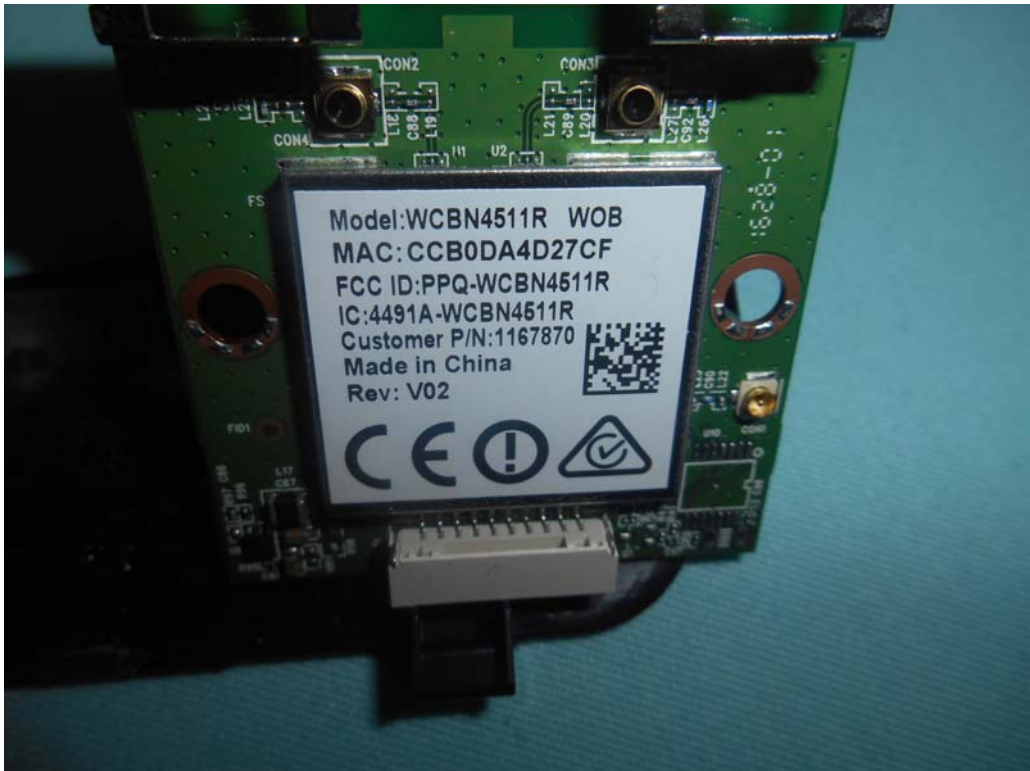
FIGURE 16 LED LCD TV (M/N: LC-50N6000U) RF BOARD LABEL
