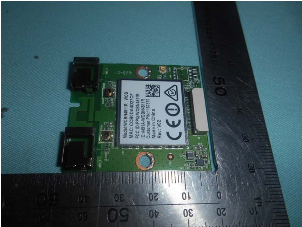
FIGURE 13 LED LCD TV (M/N: LC-50N6000U) RF BOARD (COMPONENT SIDE)
