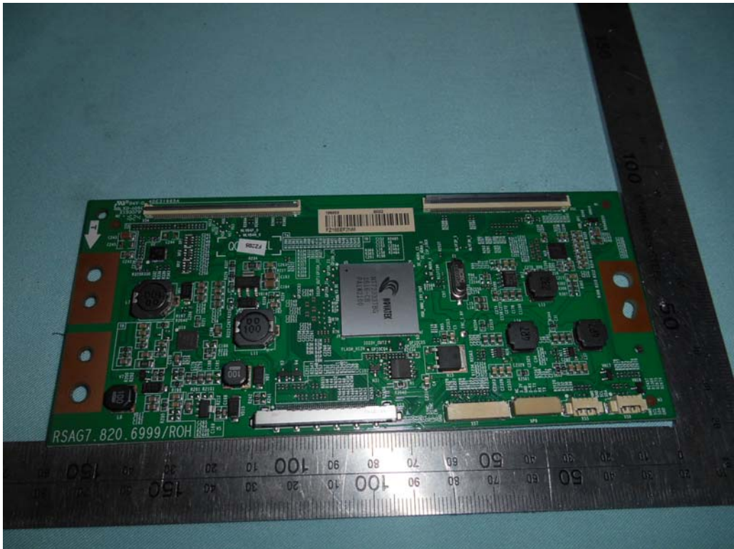
FIGURE 10 LED LCD TV (M/N: LC-50N6000U) PANEL BOARD (COMPONENT SIDE)
