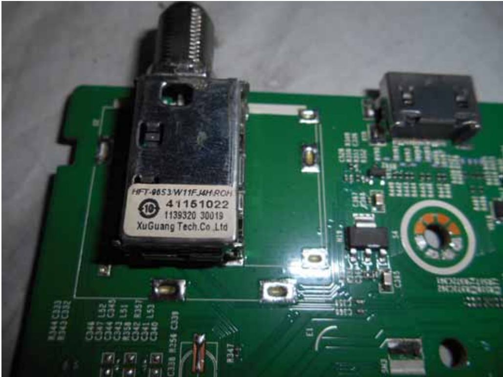
FIGURE 6 LED LCD TV (M/N: LC-65N5200U) TUNER
