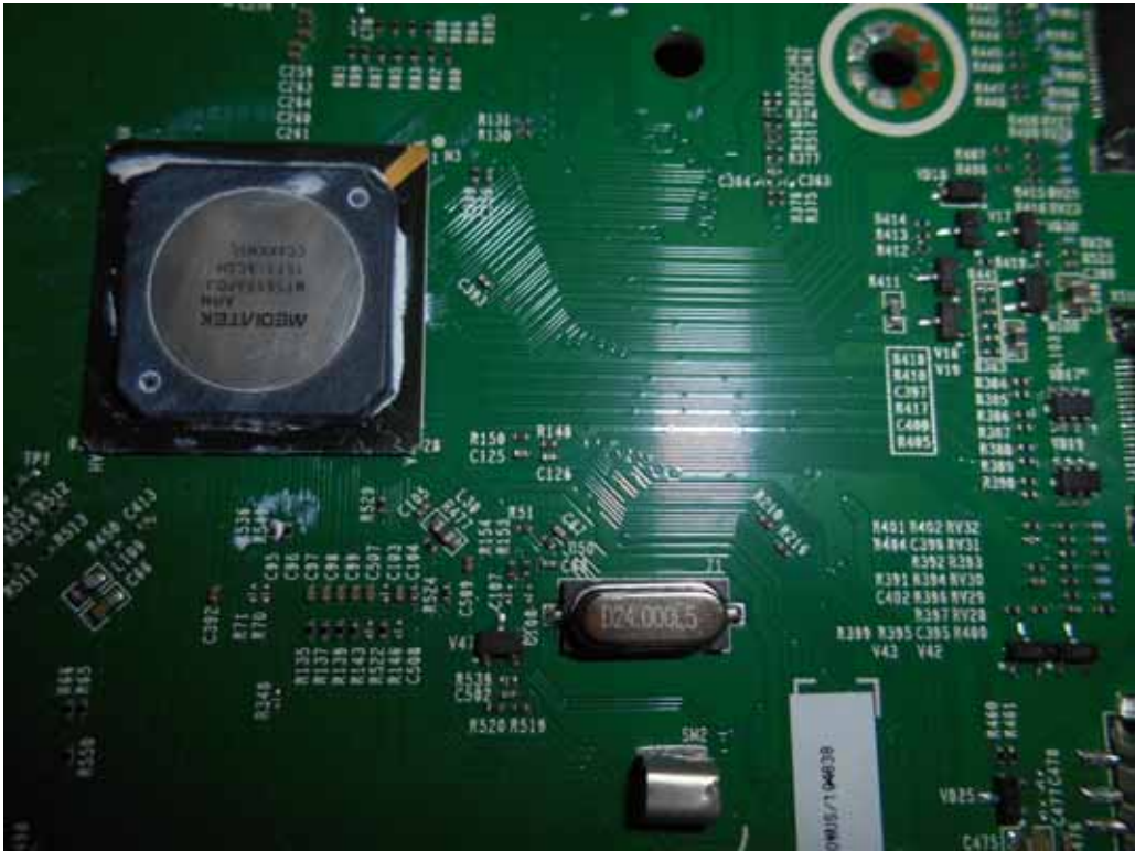
FIGURE 5 LED LCD TV (M/N: LC-65N5200U) CHIP#1 & CRYSTAL#1 ON MAIN BOARD
