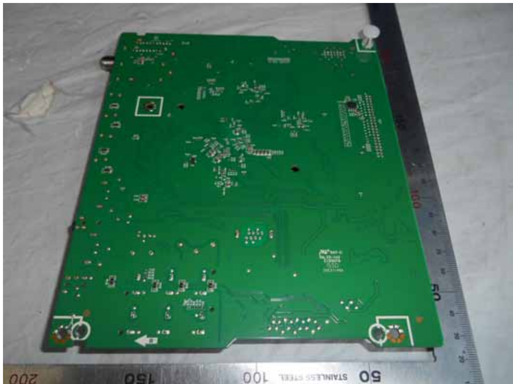
FIGURE 4 LED LCD TV (M/N: LC-65N5200U) MAIN BOARD (SOLDERED SIDE)
