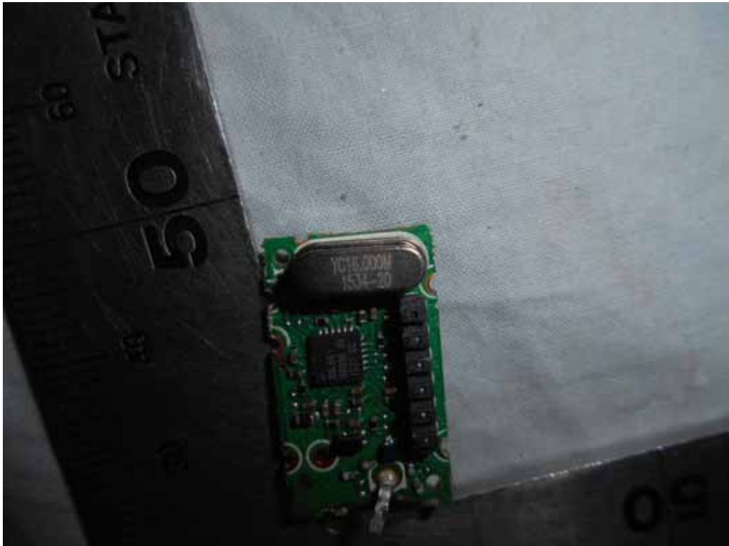
FIGURE 9 LED LCD TV (M/N: LC-65N5200U) CHIP & CRYSTAL ON TUNER BOARD
