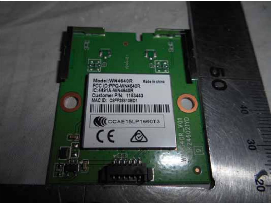
FIGURE 12 LED LCD TV (M/N: LC-65N5200U) RF BOARD LABEL
