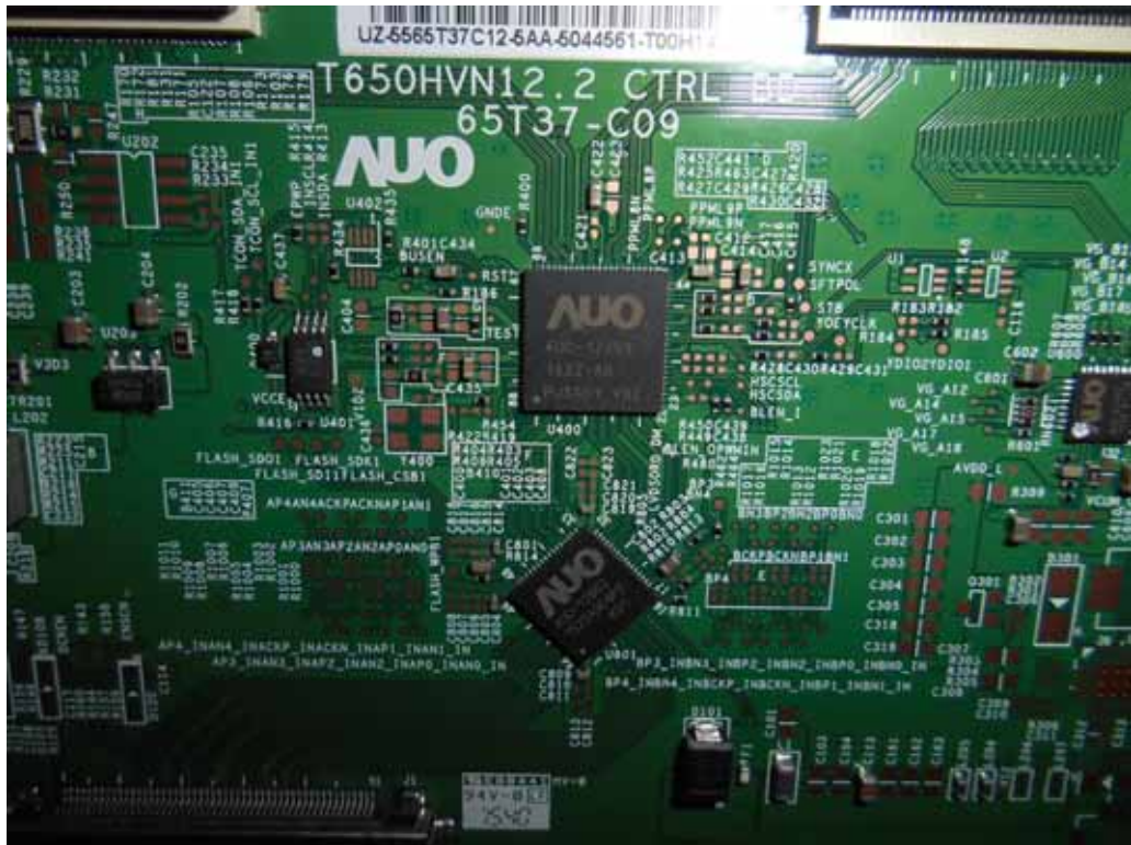
FIGURE 21 LED LCD TV (M/N: LC-65N5200U) CHIP & CRYSTAL ON PANEL BOARD
