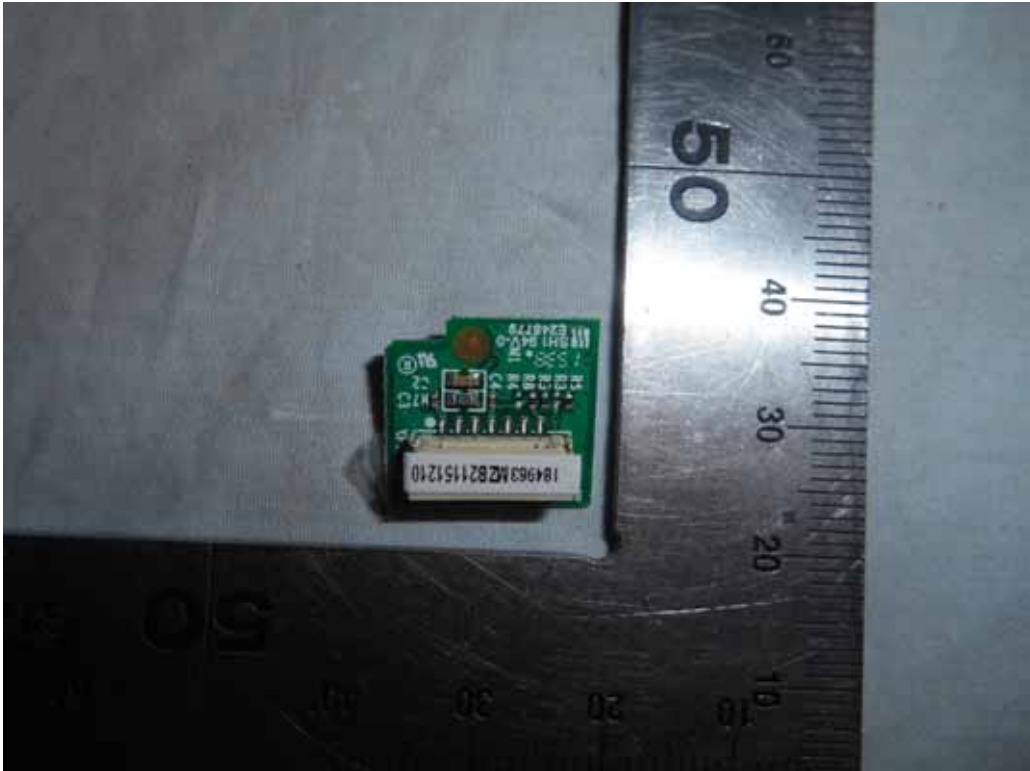
FIGURE 16 LED LCD TV (M/N: LC-65N5200U) IR BOARD (SOLDERED SIDE)
