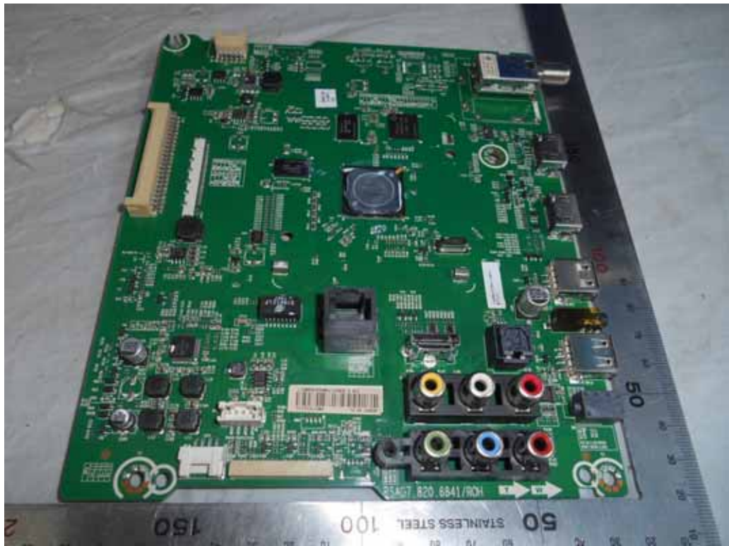
FIGURE 3 LED LCD TV (M/N: LC-65N5200U) MAIN BOARD (COMPONENT SIDE)
