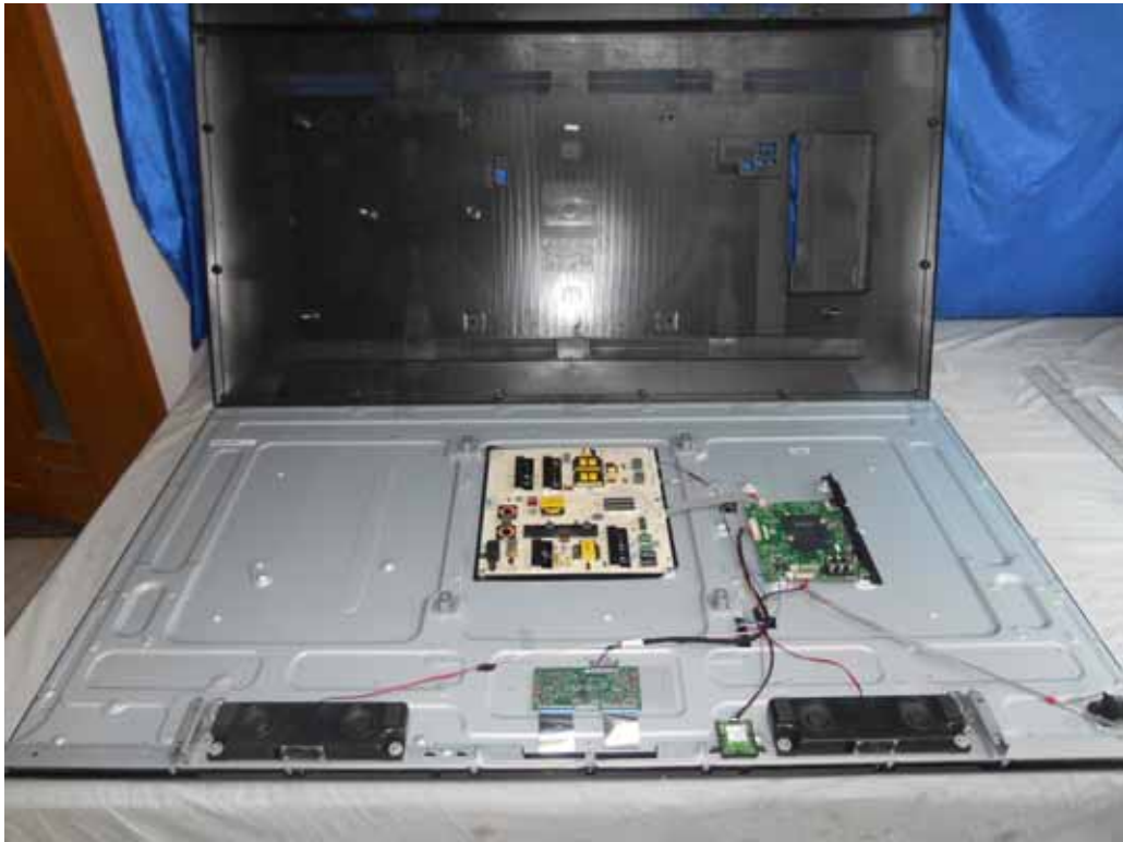
FIGURE 1 LED LCD TV (M/N: LC-65N5200U) COVER REMOVED
