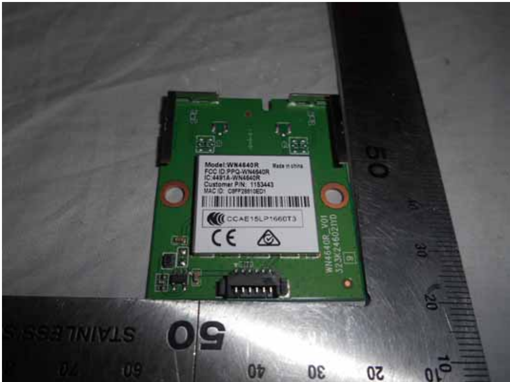
FIGURE 10 LED LCD TV (M/N: LC-65N5200U) RF BOARD (COMPONENT SIDE)
