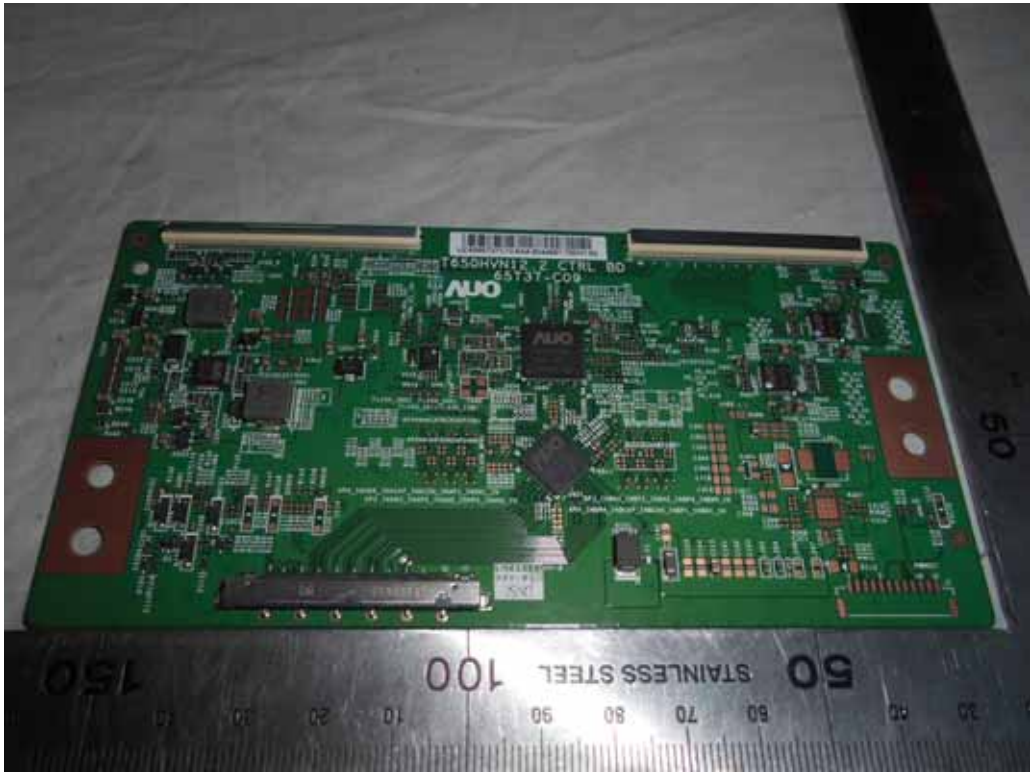
FIGURE 19 LED LCD TV (M/N: LC-65N5200U) PANEL BOARD (COMPONENT SIDE)
