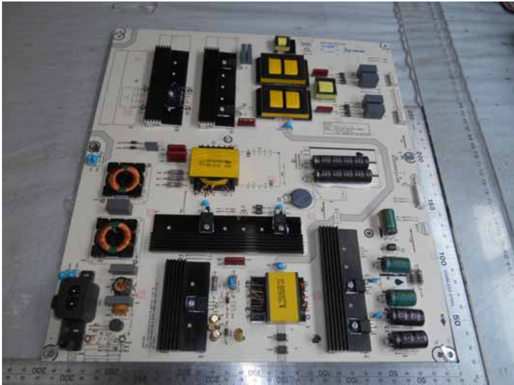
FIGURE 17 LED LCD TV (M/N: LC-65N5200U) POWER BOARD (COMPONENT SIDE)
