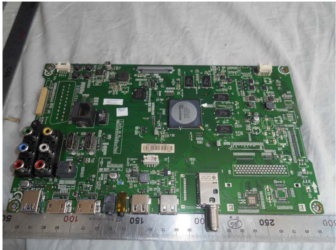
FIGURE 5 LED LCD TV (M/N: LC-65N7000U) MAIN BOARD (COMPONENT SIDE)
