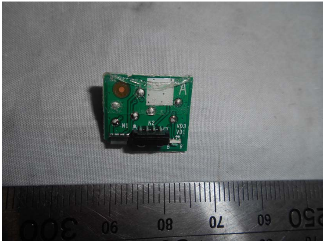
FIGURE 20 LED LCD TV (M/N: LC-65N7000U) IR BOARD (COMPONENT SIDE)
