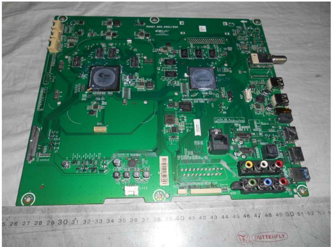
FIGURE 3 LED LCD TV (M/N: LTDN75K700GUWUS) MAIN BOARD (COMPONENT SIDE)
