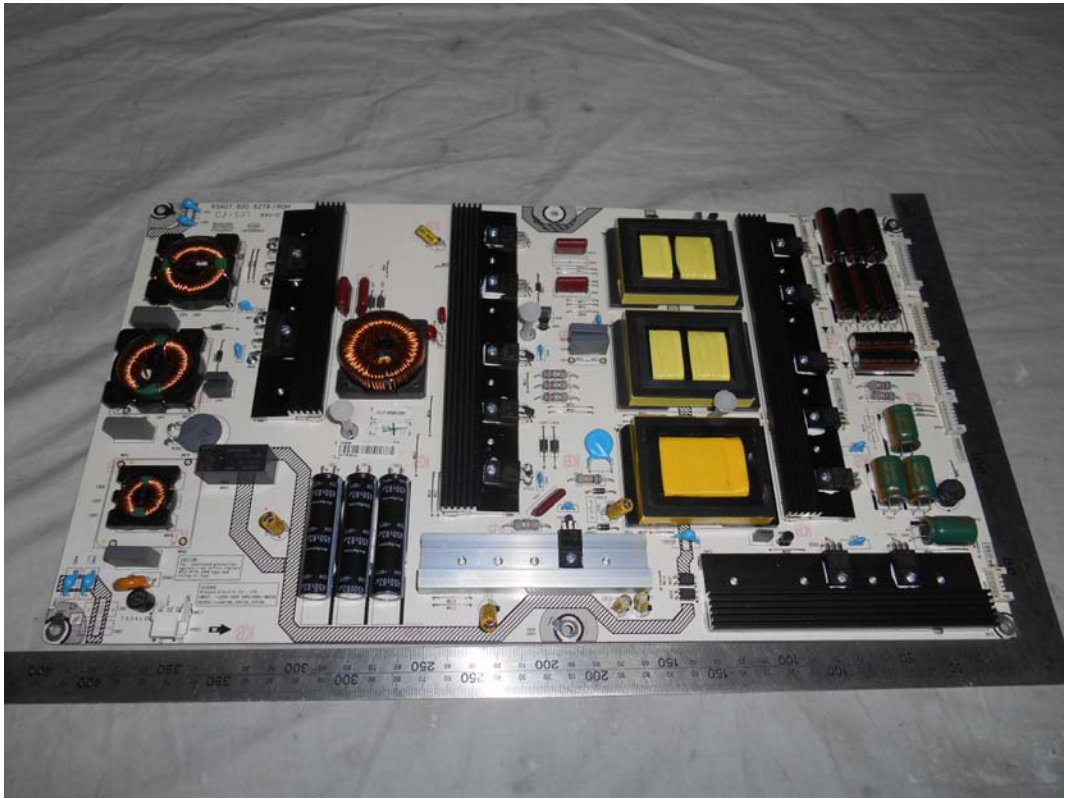
FIGURE 18 LED LCD TV (M/N: LTDN75K700GUWUS) POWER BOARD (COMPONENT SIDE)
