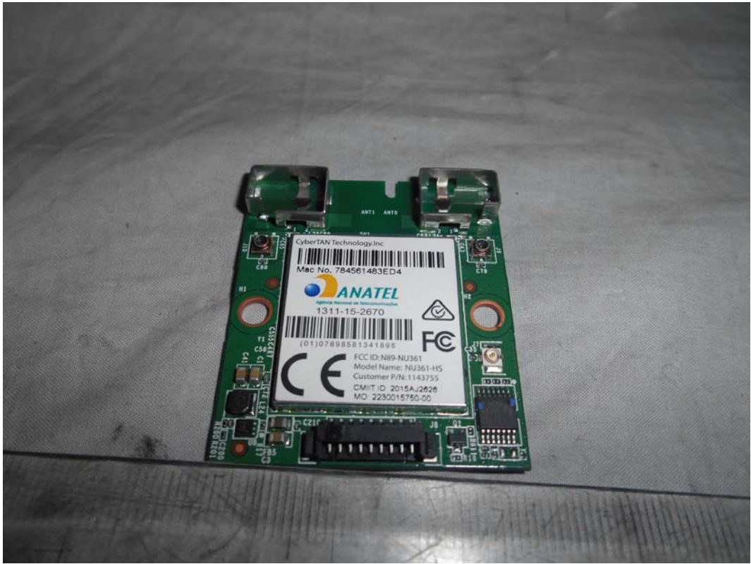
FIGURE 15 LED LCD TV (M/N: LTDN75K700GUWUS) RF BOARD (COMPONENT SIDE)
