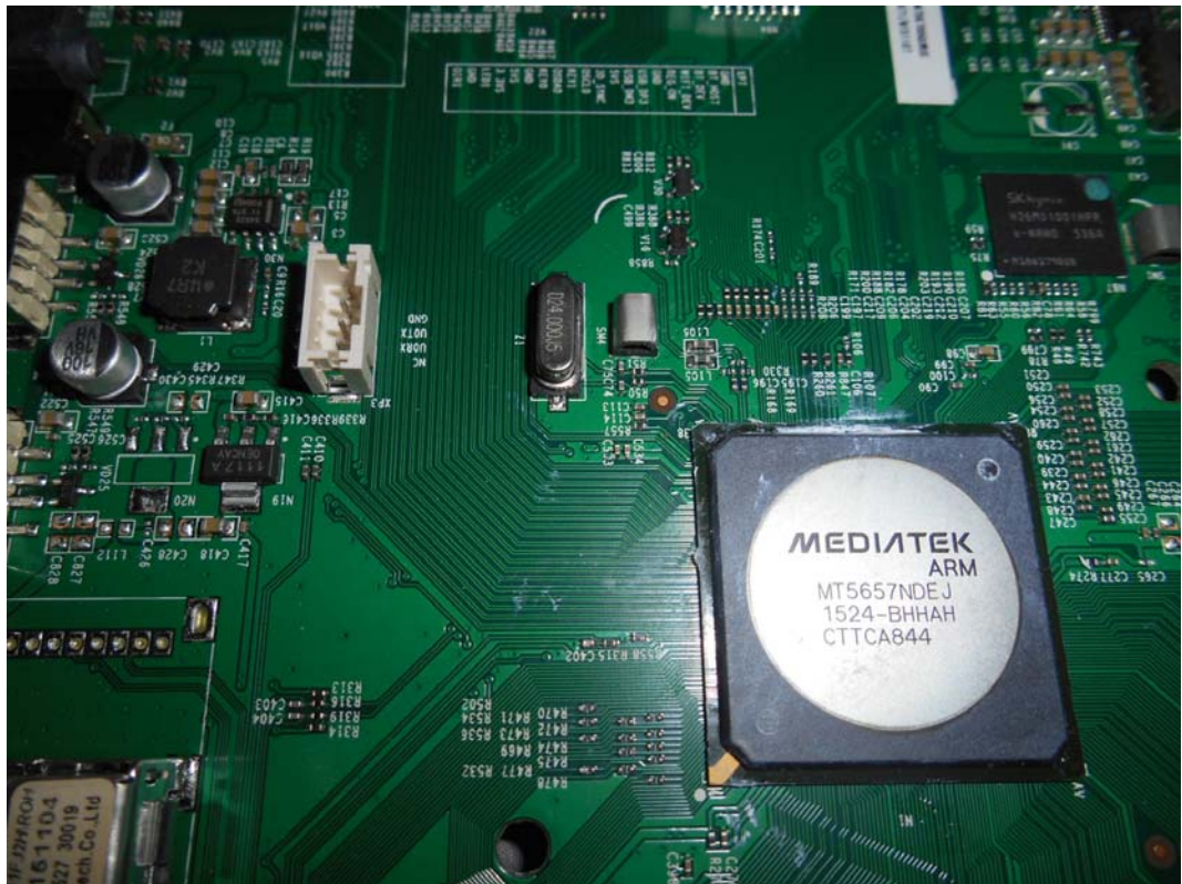
FIGURE 5 LED LCD TV (M/N: LTDN75K700GUWUS) CHIP & CRYSTAL#1 ON MAIN BOARD
