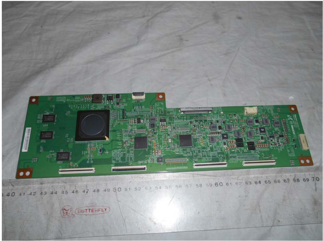
FIGURE 10 LED LCD TV (M/N: LTDN75K700GUWUS) PANEL BOARD (COMPONENT SIDE)
