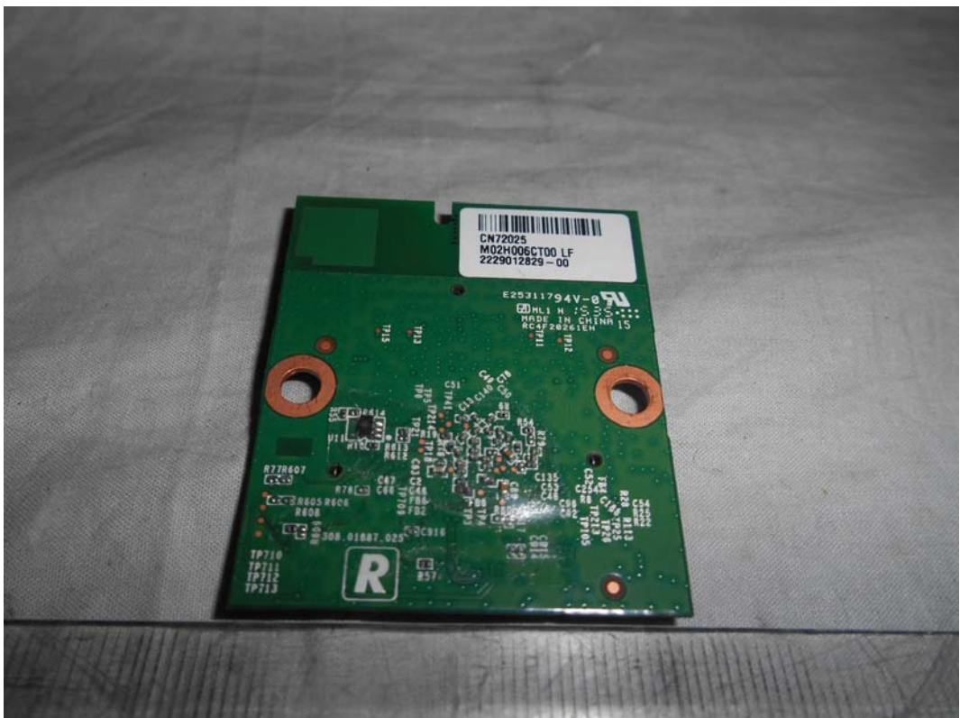
FIGURE 16 LED LCD TV (M/N: LTDN75K700GUWUS) RF BOARD (SOLDERED SIDE)
