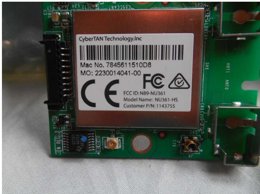
FIGURE 14 LED LCD TV (M/N: 65H7B) LABEL OF RF BOARD
