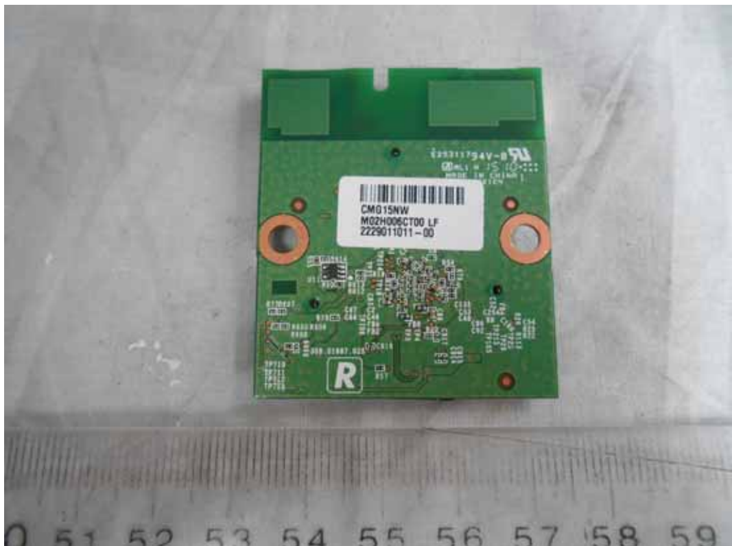
FIGURE 13 LED LCD TV (M/N: 65H10B) RF BOARD (SOLDERED SIDE)
