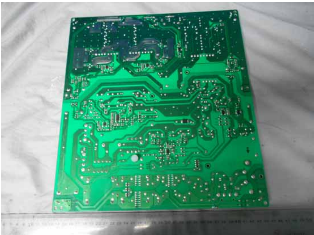
FIGURE 11 LED LCD TV (M/N: 65H10B) POWER BOARD (SOLDERED SIDE)
