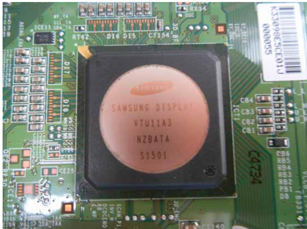
FIGURE 18 LED LCD TV (M/N: 65H10B) CHIP ON SIGNAL BOARD #1
