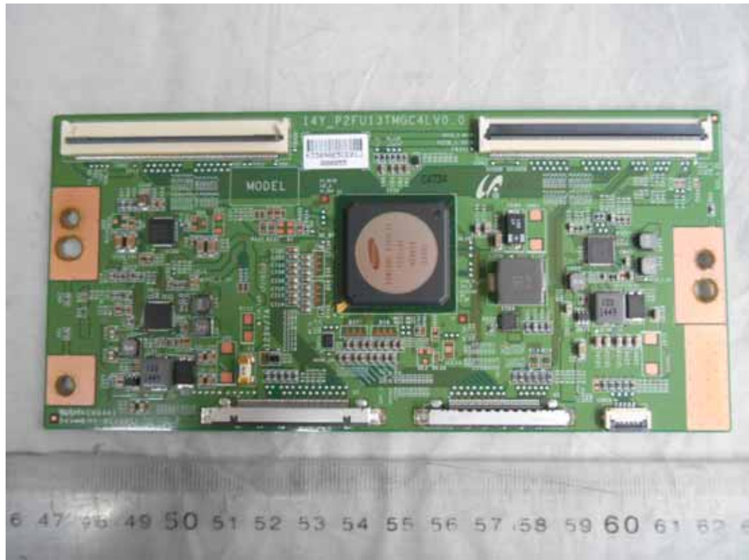
FIGURE 16 LED LCD TV (M/N: 65H10B) SIGNAL BOARD #1 (COMPONENT SIDE)
