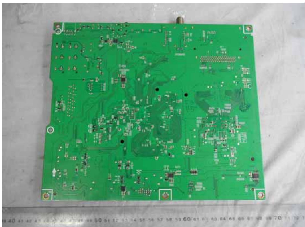
FIGURE 4 LED LCD TV (M/N: 65H10B) MAIN BOARD (SOLDERED SIDE)
