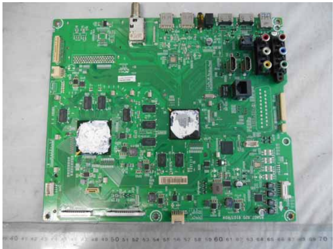
FIGURE 3 LED LCD TV (M/N: 65H10B) MAIN BOARD (COMPONENT SIDE)
