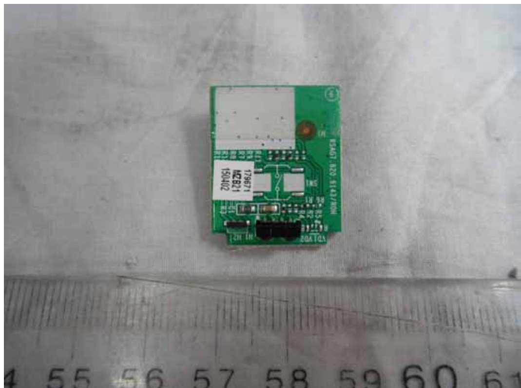
FIGURE 24 LED LCD TV (M/N: 65H10B) INTERFACE BOARD (COMPONENT SIDE)
