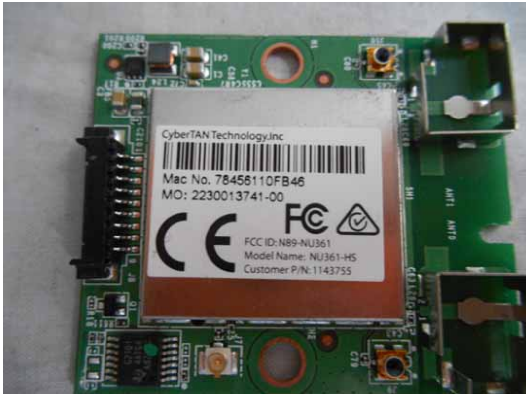
FIGURE 14 LED LCD TV (M/N: 65H10B) RF BOARD LABEL
