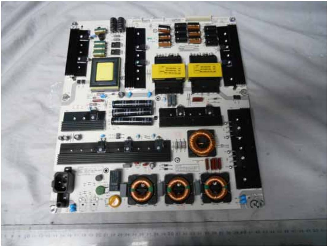
FIGURE 10 LED LCD TV (M/N: 65H10B) POWER BOARD (COMPONENT SIDE)
