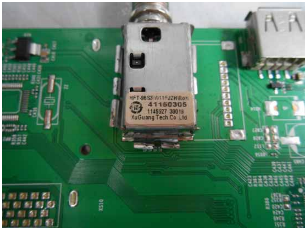
FIGURE 8 LED LCD TV (M/N: 65H10B) TUNER
