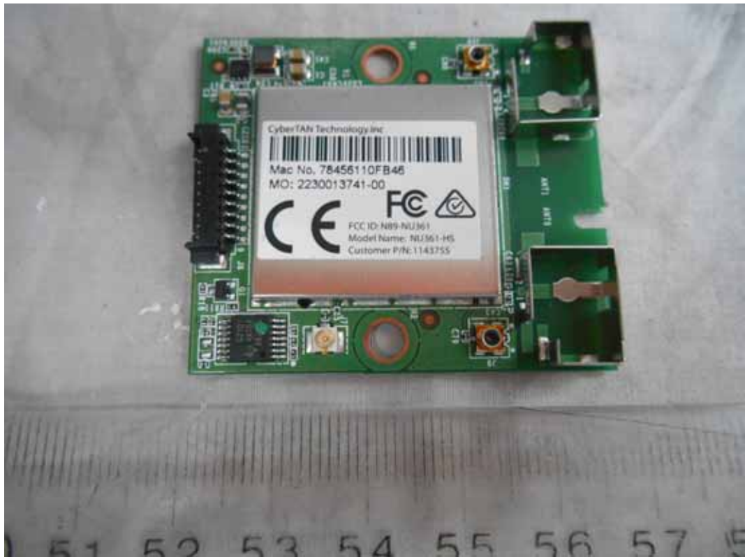
FIGURE 12 LED LCD TV (M/N: 65H10B) RF BOARD (COMPONENT SIDE)
