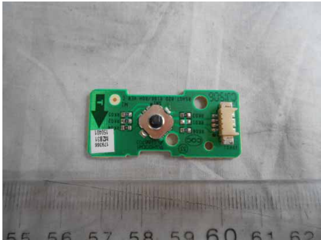
FIGURE 21 LED LCD TV (M/N: 65H10B) IR BOARD (COMPONENT SIDE)
