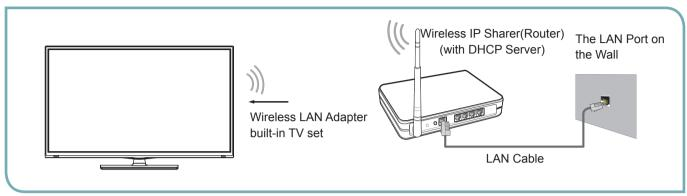
Hisense's built-in Wireless LAN Adapter supports the IEEE 802.11 b/g/n communication protocols. Hisense recommends using IEEE 802.11n router. When you play the video over a IEEE 802.11b/g connection, the video may not play smoothly.
