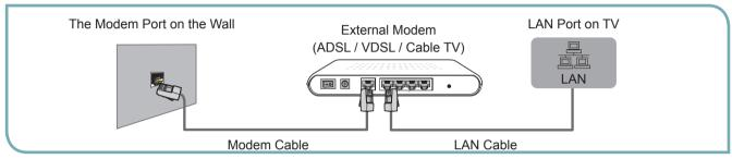
You can attach your TV to your LAN by connecting the LAN port on the back of your TV to an IP Sharer which is connected
