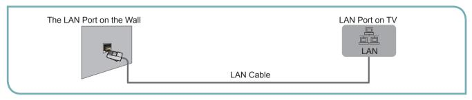
If you have a Dynamic Network, you should use an ADSL modem or router that supports Dynamic Host Configuration Protocol (DHCP). Modems and routers that support DHCP automatically provide the IP address, subnet mask, gateway, and DNS, so you don't have to enter them manually. Most home networks are Dynamic Networks.
