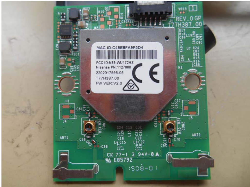
FIGURE 14 LED LCD TV (M/N: LTDN50K220WUS) RF BOARD (COMPONENT SIDE)
