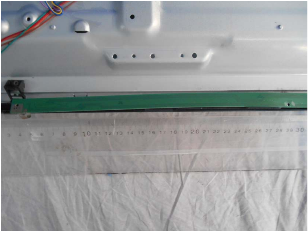
FIGURE 27 LED LCD TV (M/N: LTDN50K220WUS) CONTROL BOARD #1 (SOLDERED SIDE)
