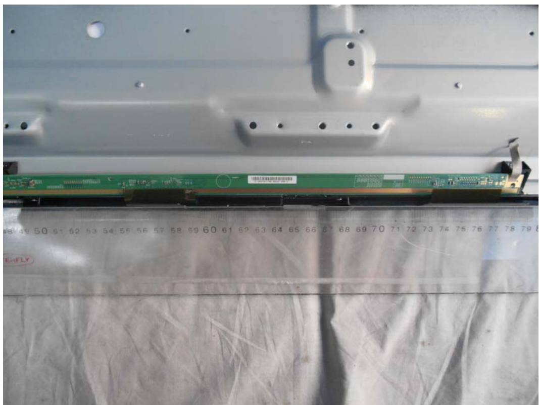
FIGURE 26 LED LCD TV (M/N: LTDN50K220WUS) CONTROL BOARD #4 (COMPONENT SIDE)
