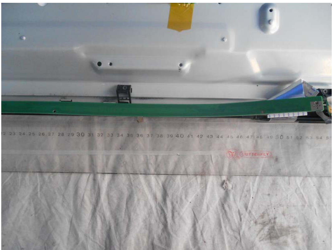
FIGURE 28 LED LCD TV (M/N: LTDN50K220WUS) CONTROL BOARD #2 (SOLDERED SIDE)
