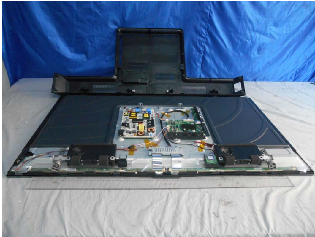
FIGURE 6 LED LCD TV (M/N: LTDN50K220WUS) COVER REMOVED
