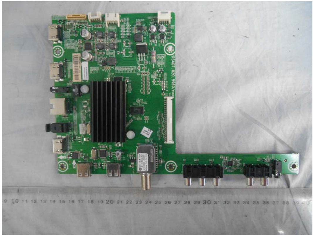
FIGURE 8 LED LCD TV (M/N: LTDN50K220WUS) MAIN BOARD (COMPONENT SIDE)
