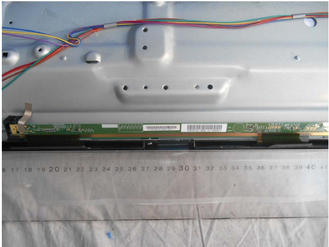
FIGURE 23 LED LCD TV (M/N: LTDN50K220WUS) CONTROL BOARD #1 (COMPONENT SIDE)
