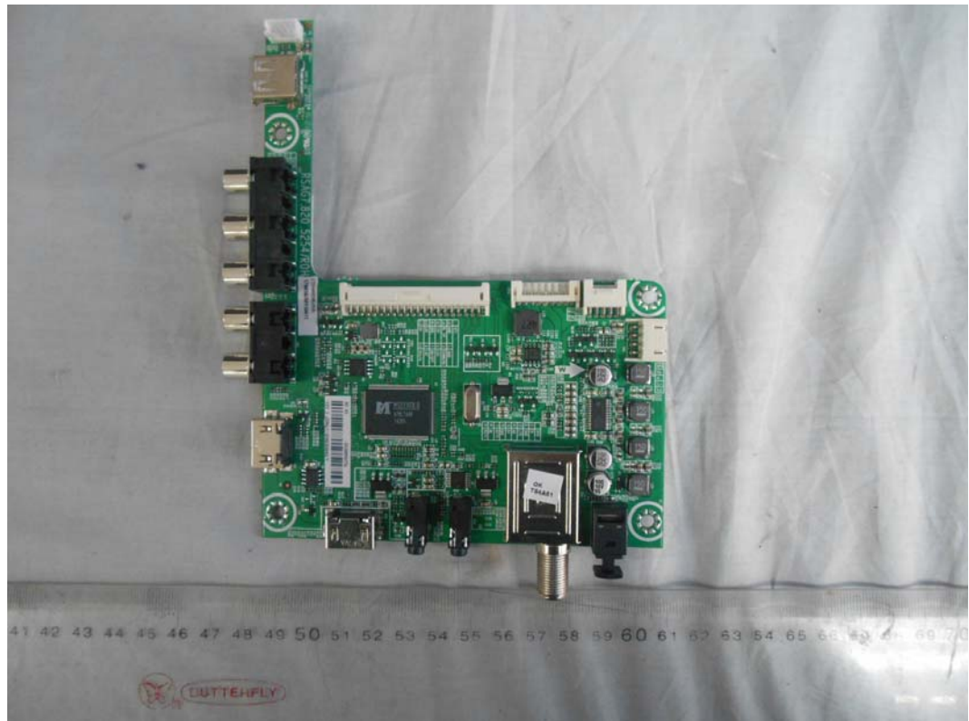
FIGURE 3 LED LCD TV (M/N: LTDN50D36US) MAIN BOARD (COMPONENT SIDE)
