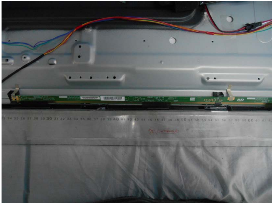
FIGURE 13 LED LCD TV (M/N: LTDN50D36US) CONTROL BOARD #1 (COMPONENT SIDE)
