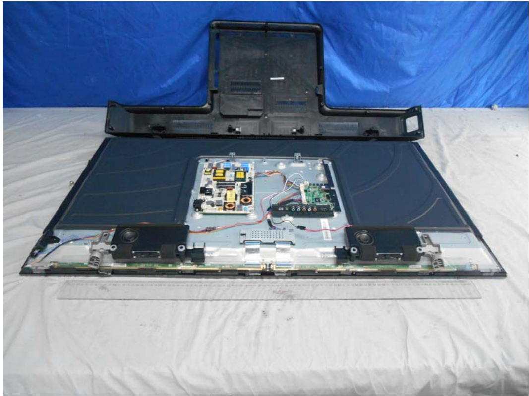
FIGURE 1 LED LCD TV (M/N: LTDN50D36US) COVER REMOVED #1
