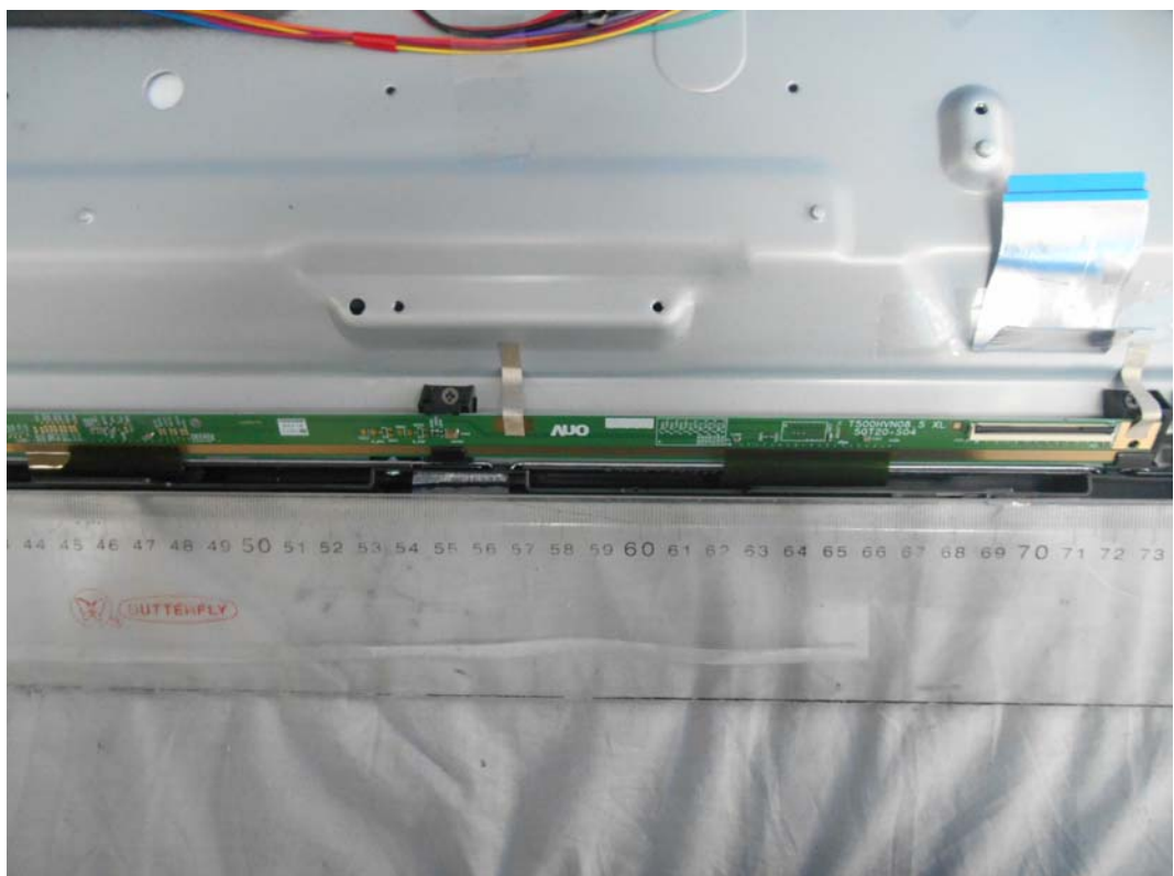
FIGURE 14 LED LCD TV (M/N: LTDN50D36US) CONTROL BOARD #2 (COMPONENT SIDE)
