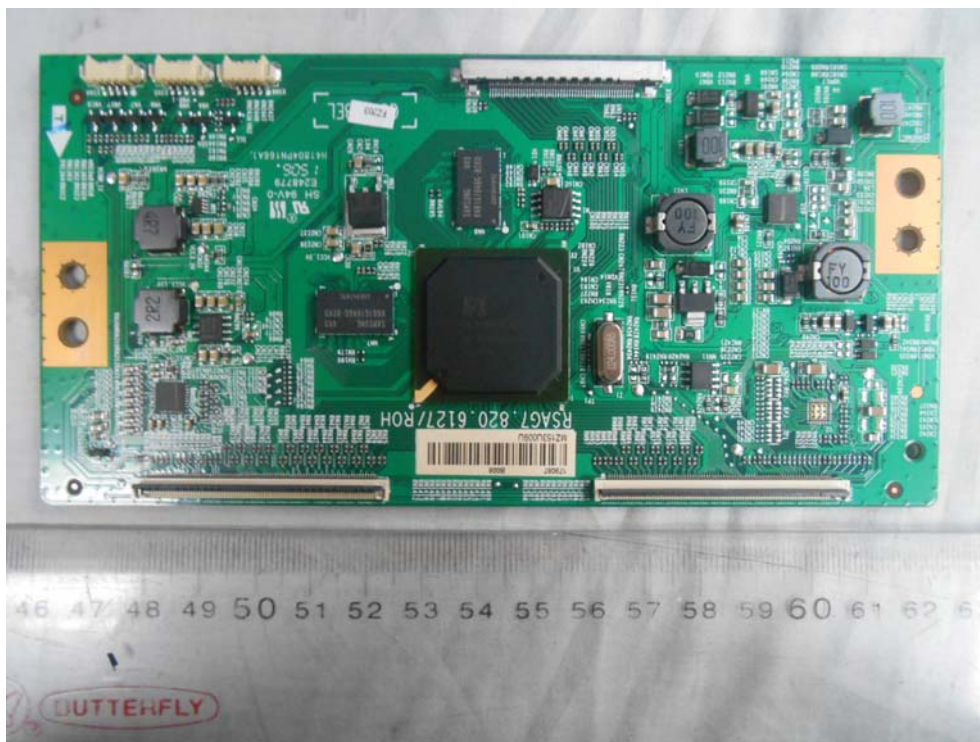
M/N: HD550DU-B51\S3.B2\ROH PANEL BOARD (COMPONENT SIDE)
