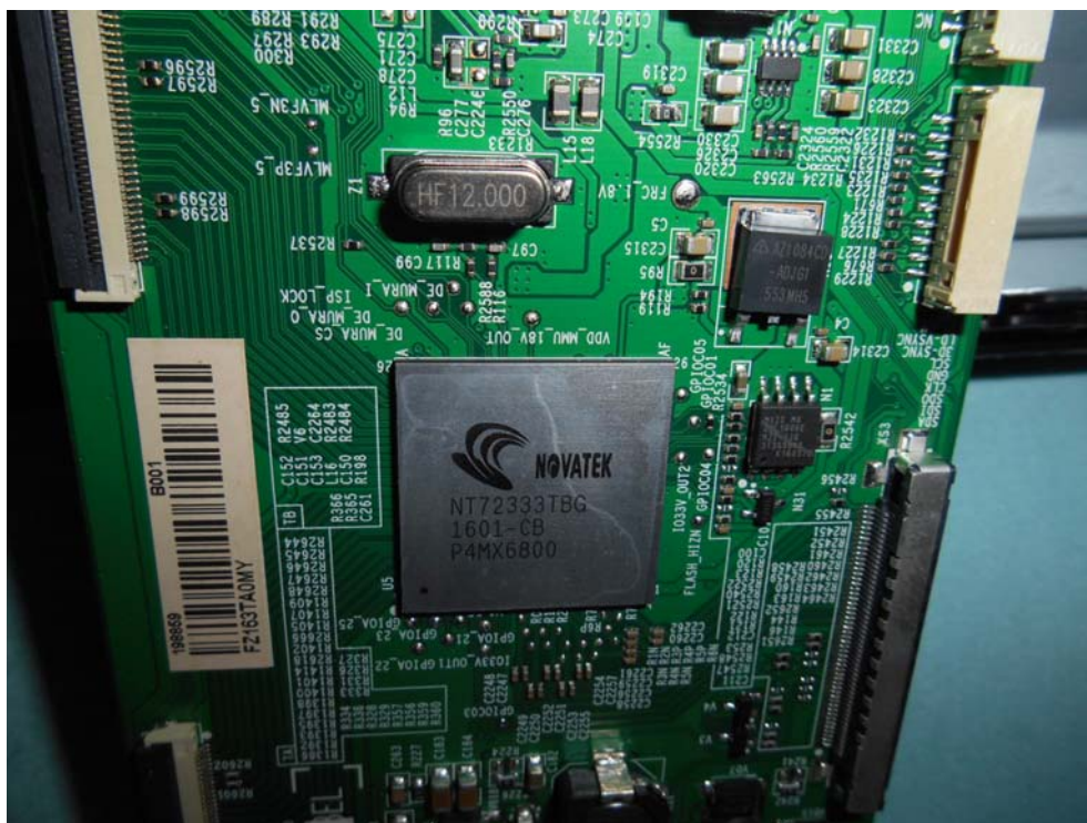
M/N: HD550DU-B51 (010) CHIP & CRYSTAL ON PANEL BOARD
