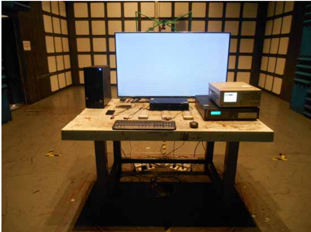
FRONT VIEW OF RADIATED EMISSION TEST (BEIOW 1GHZ)
