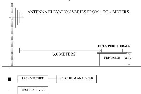
4.2.2 Radiated emission test setup
