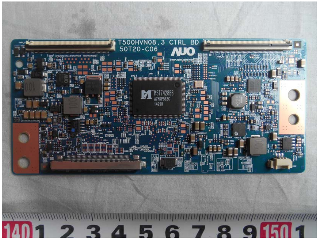
FIGURE 15 LED LCD TV (M/N: 50H5GB) SIGNAL BOARD (COMPONENT SIDE)
