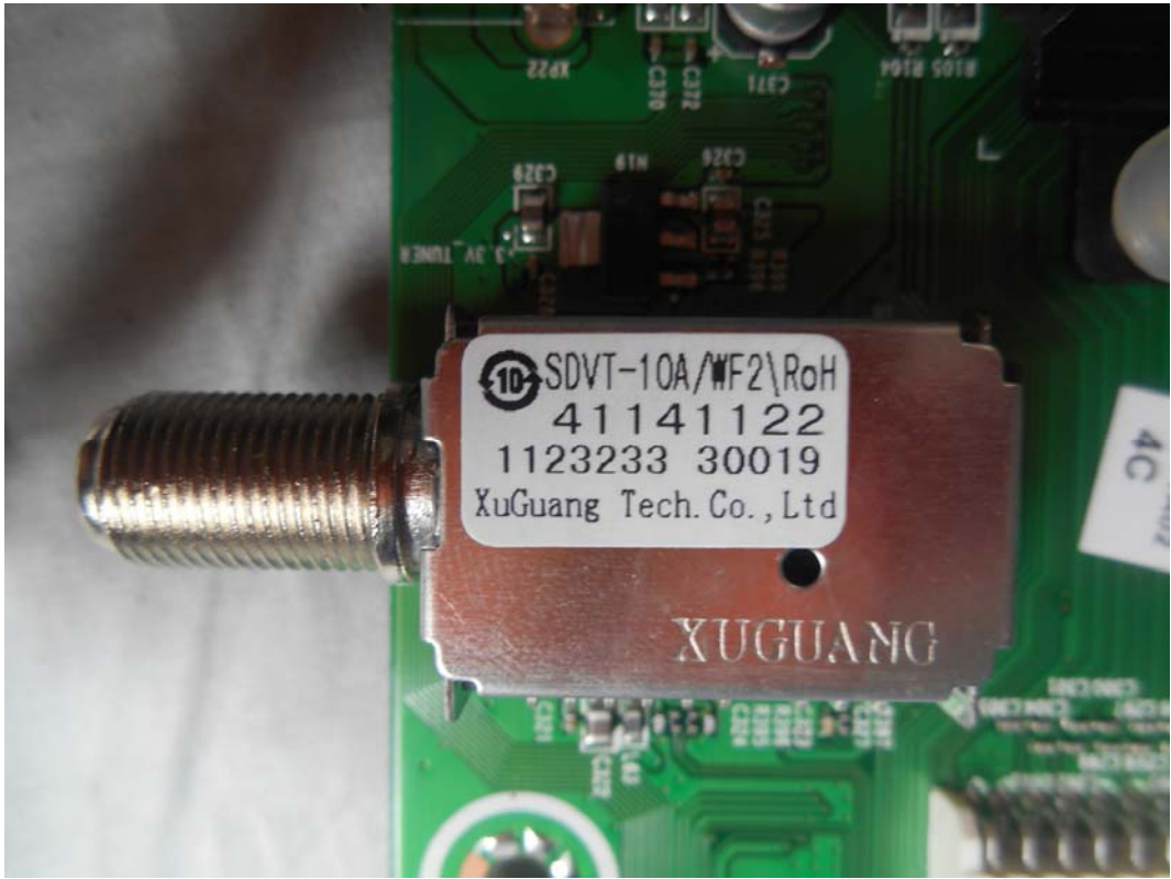
FIGURE 8 LED LCD TV (M/N: 50H5GB) TUNER ON MAIN BOARD
