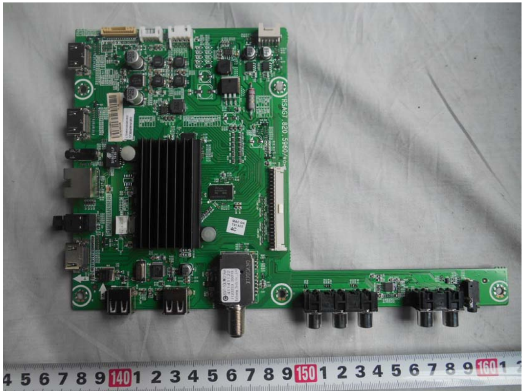
FIGURE 4 LED LCD TV (M/N: 50H5GB) MAIN BOARD (COMPONENT SIDE)
