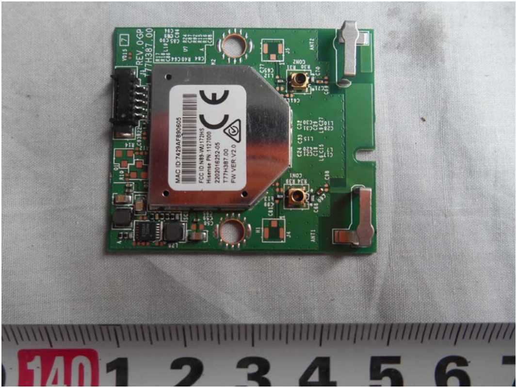
FIGURE 12 LED LCD TV (M/N: 50H5GB) RF BOARD (COMPONENT SIDE)
