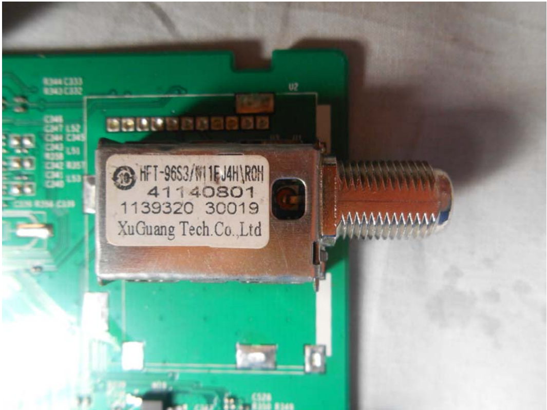
FIGURE 7 LED LCD TV (M/N: 55H6B) TUNER ON MAIN BOARD
