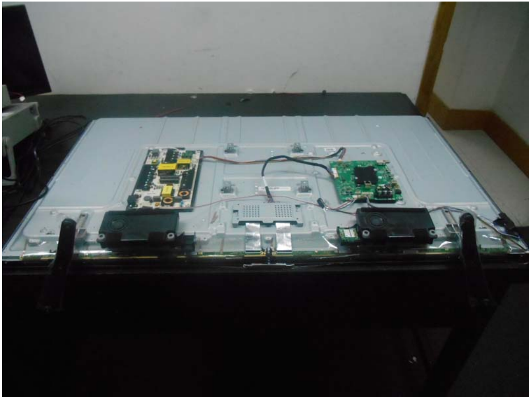
FIGURE 1 LED LCD TV (M/N: 55H6B) COVER REMOVED
