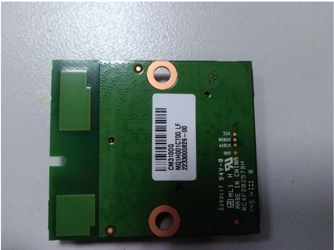
FIGURE 12 LED LCD TV (M/N: 55H6B) RF BOARD (SOLDERED SIDE)
