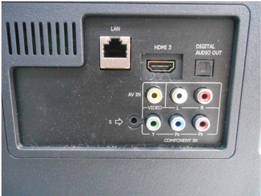
FIGURE 3 LED LCD TV (M/N: 55H6B) PORTS #1
