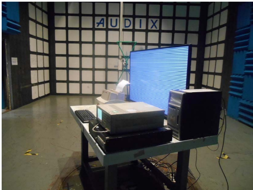
SETUP WITH MAXIMUM DETECTED EMISSION AT VERTICAL POLARIZATION (TEST MODE: HDMI 640*480@60Hz & 1kHz PLAYING)
