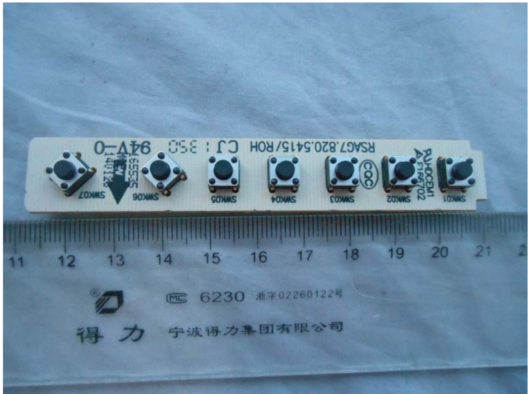
FIGURE 12 LED LCD TV (M/N: 55H7EG) KEY BOARD (COMPONENT SIDE)
