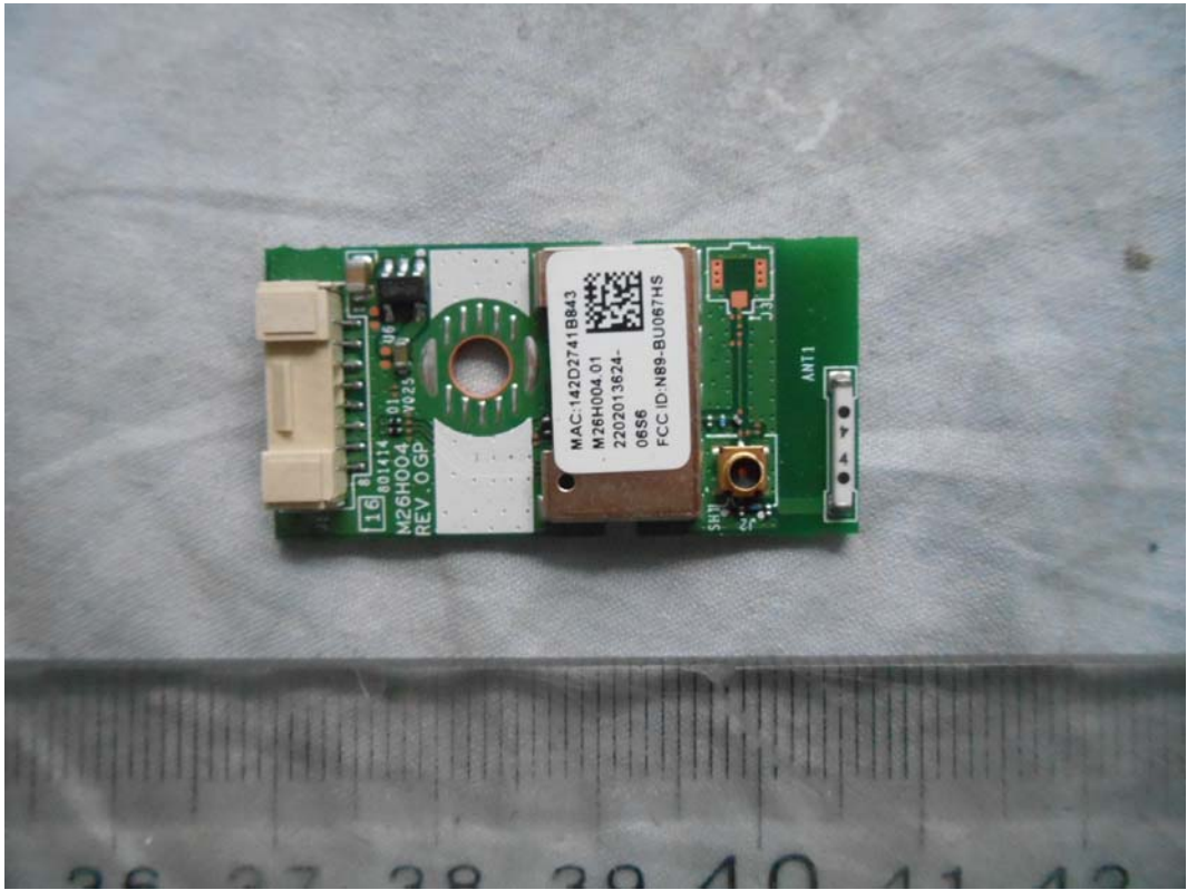
FIGURE 16 LED LCD TV (M/N: 55H7EG) RF BOARD #1 (COMPONENT SIDE)
