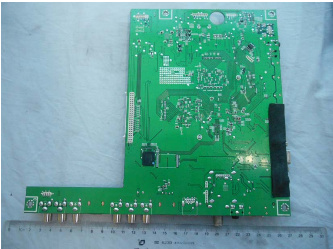
FIGURE 6 LED LCD TV (M/N: 55H7EG) MAIN BOARD (SOLDERED SIDE)
