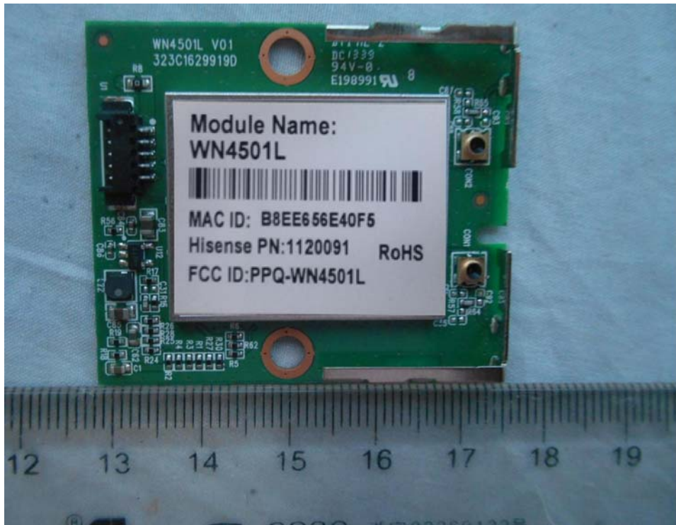
FIGURE 18 LED LCD TV (M/N: 55H7EG) RF BOARD #2 (COMPONENT SIDE)
