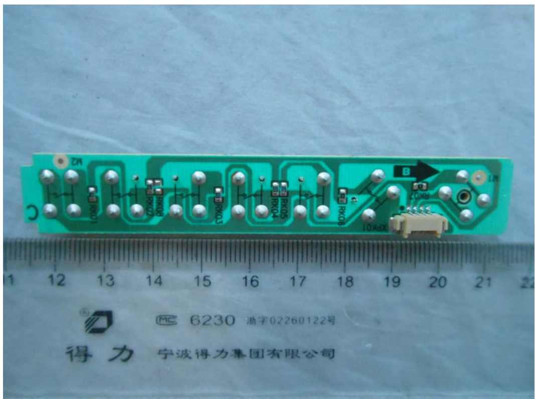
FIGURE 13 LED LCD TV (M/N: 55H7EG) KEY BOARD (SOLDERED SIDE)
