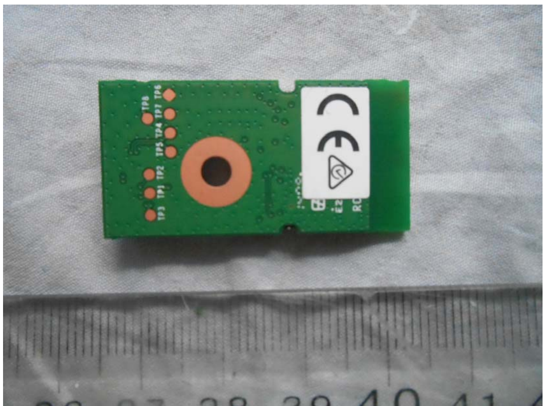
FIGURE 14 LED LCD TV (M/N: 50H7EG) RF BOARD #1 (SOLDERED SIDE)
