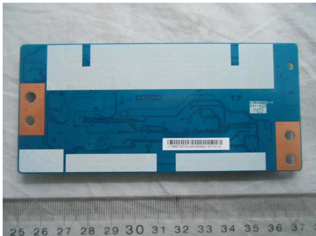
FIGURE 18 LED LCD TV (M/N: 50H7EG) LCD PANEL CONTROL BOARD (SOLDERED SIDE)
