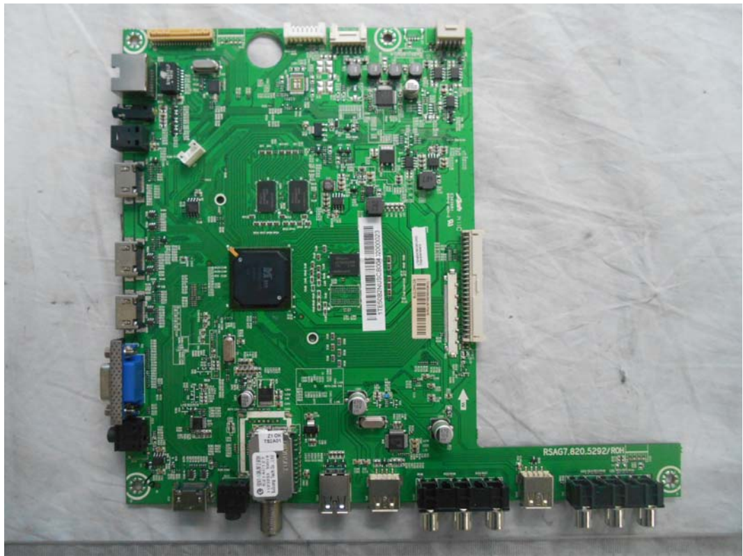
FIGURE 5 LED LCD TV (M/N: 50H7EG) MAIN BOARD (COMPONENT SIDE)
