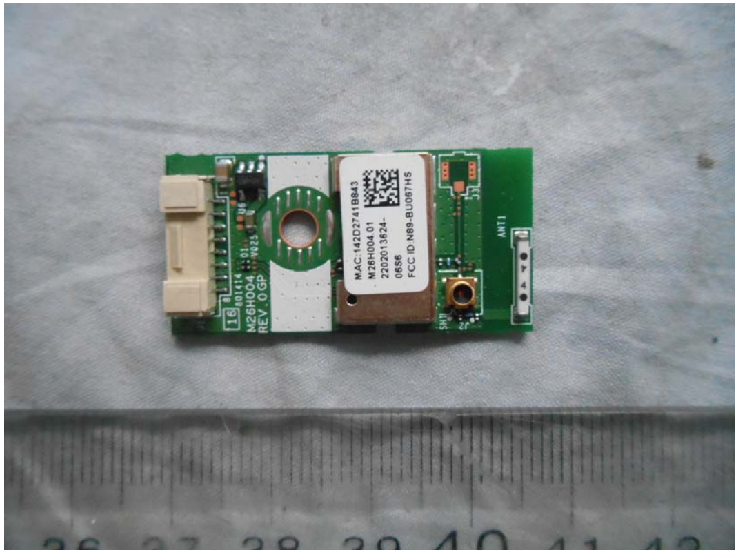
FIGURE 13 LED LCD TV (M/N: 50H7EG) RF BOARD #1 (COMPONENT SIDE)
