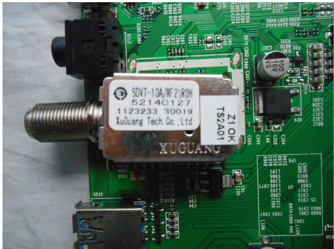
FIGURE 9 LED LCD TV (M/N: 50H7EG) TUNER ON MAIN BOARD
