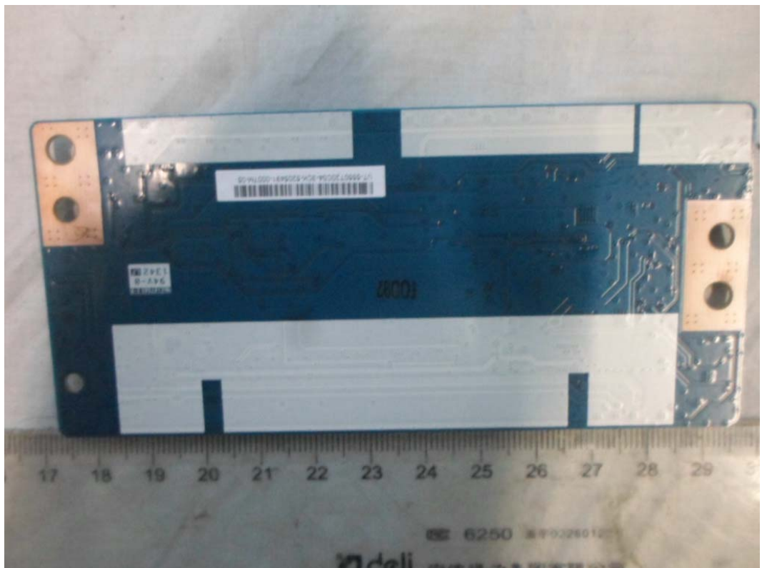
FIGURE 17 LED LCD TV (M/N: 50H4) LCD PANEL CONTROL BOARD (SOLDERED SIDE)
