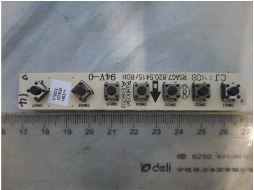
FIGURE 10 LED LCD TV (M/N: 50H4) KEY BOARD (COMPONENT SIDE)
