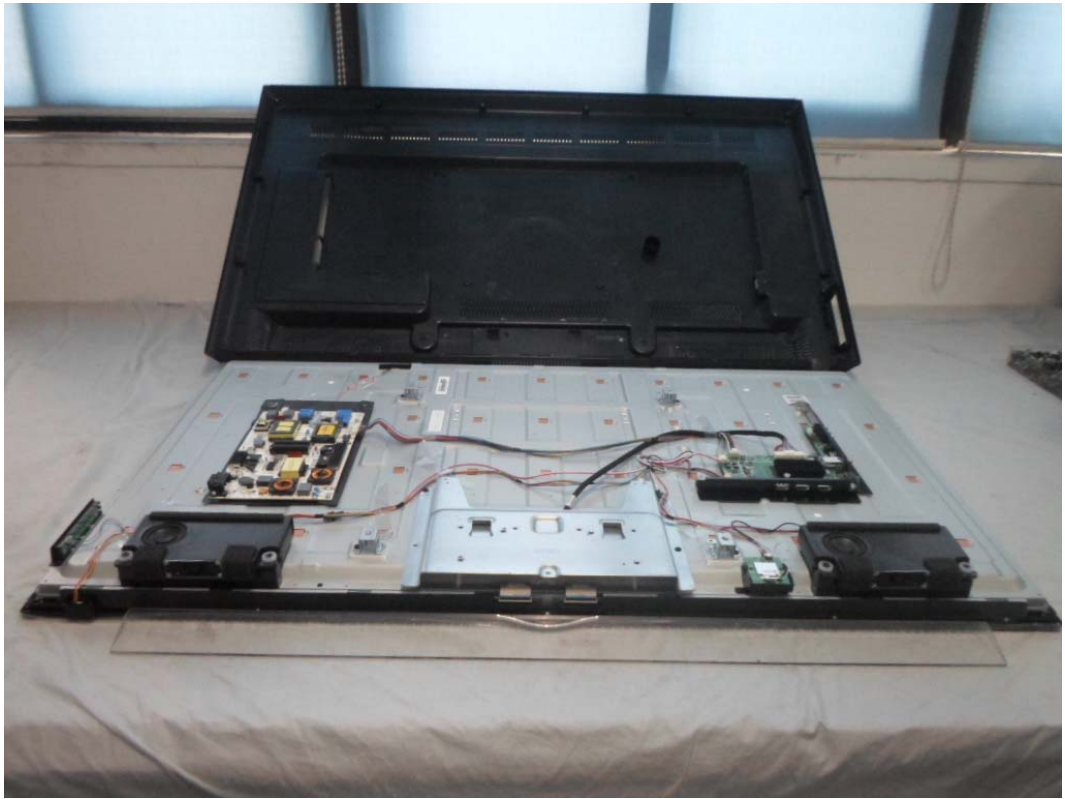
FIGURE 1 LED LCD TV (M/N: 50H4) COVER REMOVED
