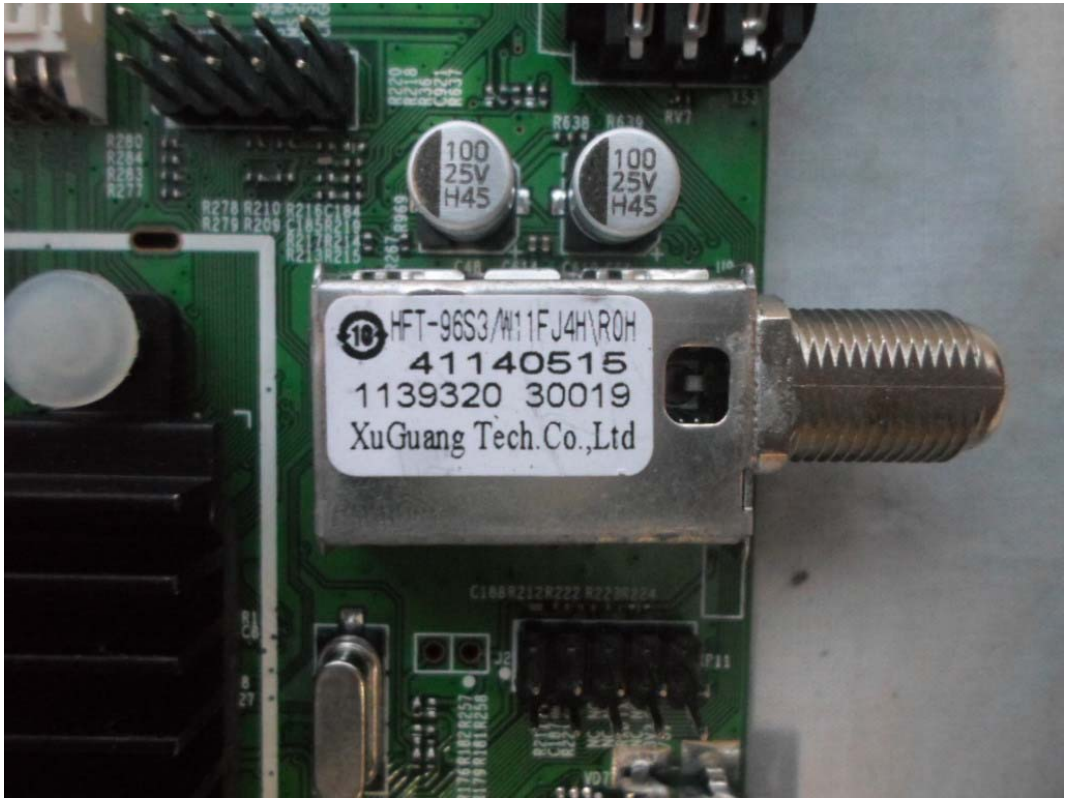
FIGURE 9 LED LCD TV (M/N: 50H4) TUNER ON MAIN BOARD
